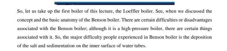
Now, see if you recall that the Benson boiler, the tube's diameter was small. So, sometimes it is advantageous, but if any sedimentation, debris or salt may get deposited over time, there may be a chance of choking. So, if this deposition is there, it will reduce the heat transfer, and ultimately the power generation or steam generation capacity would be adversely impacted.
