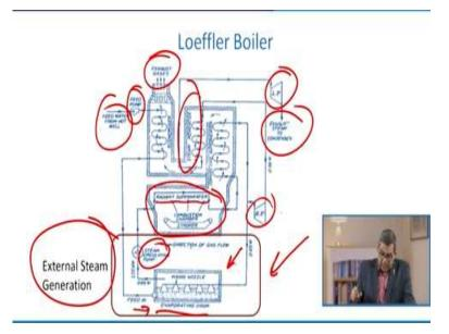
Now, is you can see the basic anatomy of the boiler or Loeffler boiler. Now, here again, I am repeating that the basic ingredient of our basic anatomy of all the boilers is similar; the only difference is the different types of parameters and configuration. Like here, you will see that exhaust, steam, high pressure, low-pressure pumps; this is the stoker type of combustion chamber. Here you will find the superradiant heaters.
