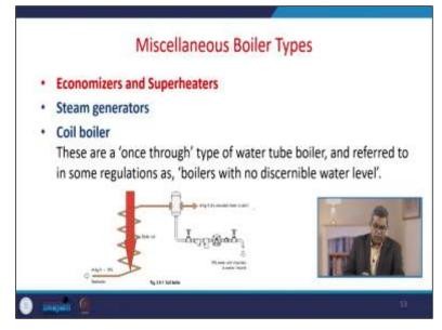
Another is the miscellaneous boiler type like coil boilers. They are a once-through type of boiler, which we have already discussed, and they are referred to some regulations with the boiler with no disclaim water level.
