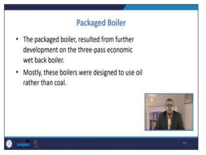
So, the packaged boiler resulted from the further development of the three past economic wet boilers mostly, and these boilers were designed to use oil rather than coal.
