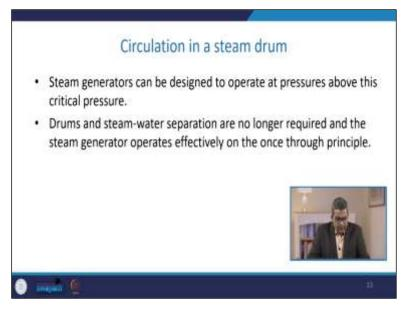
Now steam generators can be designed to operate at pressures above this critical pressure. Drums and steam-water separation are no longer required, and the steam generator operates effectively on the once-through principle.
