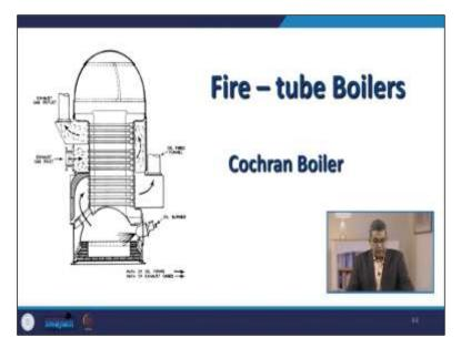
The basic points of this Cochran boiler are here this is the oil for the fired boiler. Now here is the gas inlet and gas outlet. You can see the tubes. This is the fire inside the tube, submerged in the water. So, you can produce the steam, and you can discharge the steam from here.
