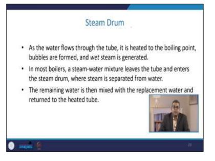
As the water flows through the tube, it is heated to the boiling point, bubbles are formed, and wet steam is generated in the boiler. The steam-water mixture leaves the tube and enters the steam drum, where steam is separated from the water. The remaining water is usually mixed with the replacement water and returned to the heated tube.
