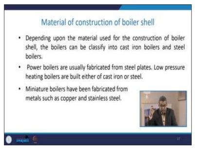
Another classification is based on the material of construction of the boiler shell. So, depending upon the material used for the construction of the boiler shell, the boilers can be classified into cast iron boilers and steel boilers. So, power boilers are usually fabricated from steel plates. Low-pressure heating boilers are built either of cast iron or steel. Sometimes miniature boilers have been fabricated from metals such as copper or stainless steel.
