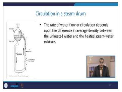
The water flow rate or circulation depends on the difference in average density between the unheated water and the heated steam-water mixture.
