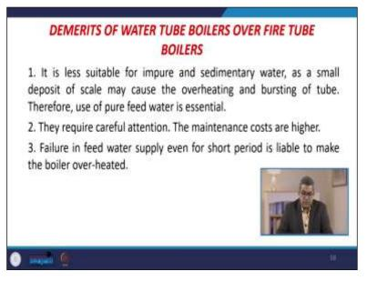
There are certain demerits of water tube boilers over fire tube boilers. They are less suitable for impure and sedimentary waters. So, the purest form of water is needed. Now, as a small deposit of scale may cause the overheating and bursting of the tube, safety may be at stake. Therefore you need to use pure feed water, which is again, you can say the economic aspect is always in there while using the purity of while considering the purity of the feed water.
