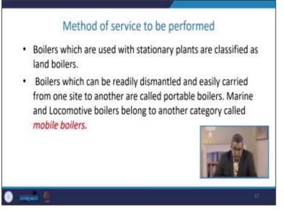
Again, we would like to discuss more this one is the service method. So, the boiler used for the stationary plant is classified as land boilers and boilers that are readily dismantled and easily carried from one side to another. They are called portable boilers, marine and locomotive boilers; we have already discussed them.
