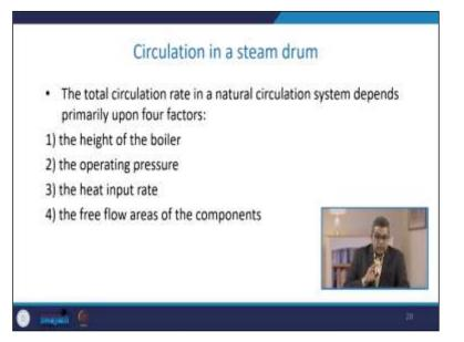
The total circulation rate in the natural system of circulation depends primarily upon four factors: what is the height of the boiler, the what is operating pressure, the third is the heat input rate, and the third is free flow area of the component.
