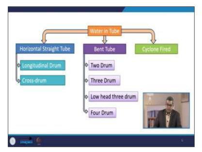
When we talk about the water and tube type of boiler, they are again divided into three categories. One is the horizontal straight tubes. This may be the longitudinal drum or a cross drum. There may be a bent tube, maybe two drums, three-drum, low head, three drums, or four drums, even they can have four drums, and a cyclone fired boilers.
