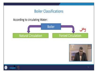
Then sometimes, people do classify based on the circulation of water concept. This boiler can now be classified in two categories: natural circulation or forced circulation. Then again, one classification may be based on the position of the principal axis. This may be either vertical horizontal, or sometimes inclined like this. Then steam pressure, we discussed the various steam classification based on the pressure.
