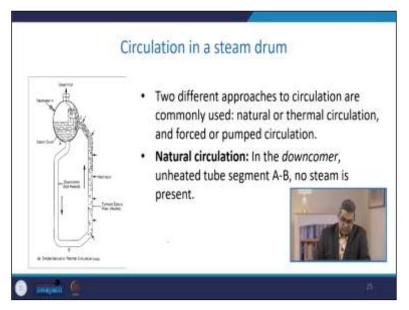
Now, two different types of approaches for circulation are attributed natural or thermal circulation and force or pump circulation. The natural circulation is the downcomer. This is the downcomer unheated tube segment. Now, this is from A to B; no steam is present; there is no steam. (Refer Slide Time: 14:12)
