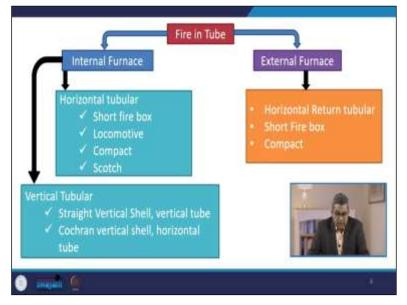
So, based on the use, one can use any boiler. Another is when we talk about the firing tube type of boiler, and they are again classified into two categories: the internally fired boilers and the externally fired boilers. There may be horizontal tubular boilers or vertical tubular boilers when
