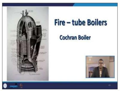
Now, this is the basic anatomy of the Cochran boiler. This is the fire-tube type of wire. You can easily see the tubes and various other mountings for this particular boiler water gauge and other types of mountings. We will discuss all these mountings in due course of time. Stop wall the steam distribution network, and This is the manhole, etc.
