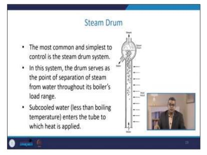
Now let us talk about the steam drum. The most common and simplest control is the steam drum type of system. Here you see that this is the steam drum in this system drum serves as the point of separation of steam from water throughout its boiler load range. We previously discussed that the water and steam both enjoy the same chamber. So, there must be a clear-cut separation system through which you can separate the steam.
