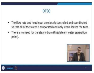
The flow rate and heat input are closely controlled and coordinated. So, all the water is evaporated, and only steam leaves the tube. So, there is no need for any kind of steam drum. Fixed steam-water separation points are there.
