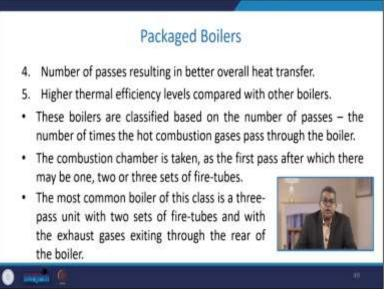
Now, with fewer passes resulting in a better overall heat transfer, you may experience a higher thermal efficiency level than other boilers. So, these boilers are classified based on the number of passes, the number of times the hot combustion gas passes through the boiler, maybe two-pass three passes, etc. So, the combustion chamber is taken as the first pass, after which there may be one or two three-set of fire tubes.
