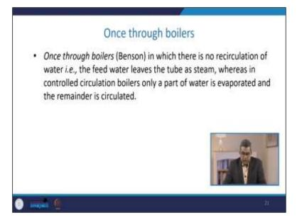
Once through boilers, the common ones to a type of boiler are the Benson boiler, in which there is no recirculation of water. The feed water leaves the tube as steam, whereas in the controlled circulation boiler, only a part of the water is evaporated, and the remainder is circulated. So, when we further elaborate on the ones through steam generators without a steam drum, you require the steam drum for other types of boilers apart from this OTSG.
