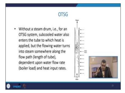
So, without a steam drum for an OTSG system, sub-cooled water also enters the tube to which heat is applied, but flowing water turns into steam somewhere along the flow path. So, this is the flow path, and you can experience the steam depending upon the water flow rate and heat input rate. So, these two are the variables for this OTSG.
