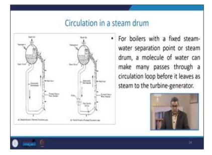
Now let us talk about the circulation in the steam drum. Now here you see that this is the steam drum steam is coming outflow water in, and here you have to have the heat input risers. This is a simple natural. Now for a system for a boiler with a fixed steam-water separation point or steam drum, a molecule of water can make many passes through a circulation loop before it leaves as steam to the turbine generator.
