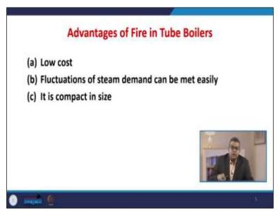
There are certain advantages attached to the fire in tube boilers: they are low cost. The fluctuation of steam demand can be met easily and is, as we discussed, it is compact.
