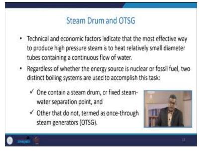
Let us talk about the steam drum and once-through type of steam generator. Now technical and economic factors indicate that the most effective way to produce high-pressure steam is to heat relatively small diameter tubes containing a continuous water flow. Whether the energy source is nuclear or fossil fuel or something else, two distinct boiling systems are used to accomplish the task.
