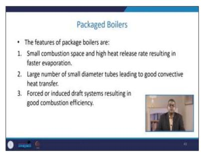
There are certain features of these packaged boilers: small combustion space and high heat release rate resulting in faster evaporation. A larger number of small diameter tubes leading to a good convective heat transfer forced or induced drop system may result in good combustion.
