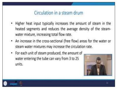
The higher heat input typically increases the amount of steam in the heated segment and reduces the steam-water mixture's average density, increasing the total flow rate. So, in this way, the total flow rate and altered. An increase in the cross-sectional, free flow area for the water or steam-water mixture may increase circulation. So, for each unit of steam produced, the amount of water entering the tube can vary from 3 to 25 units.
