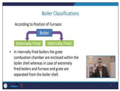
Whereas in the case of an extreme external fire boiler, the furnace and grates are separated from the boiler shell. So, suppose this is the boiler shell. So, they are separated over here in the externally fired boiler.
