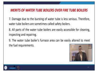
So, safety is very important. All parts of the water tube boilers are easily accessible for cleaning, inspecting, and repairing. The water tube boilers furnace area can be easily altered to meet the fuel requirement.
