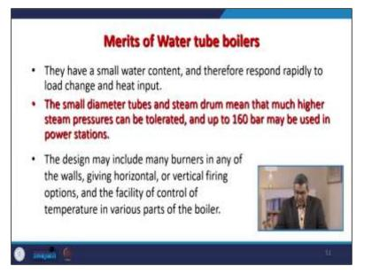
There are various merits associated with the water tube boiler. Therefore, they have small water content and respond rapidly to the load change and heat input. The small diameter tube steam diameter means much higher steam pressure. This can be tolerated, and up to 160 bars may be used in the various power station. So, the design may include many burners in any wall, giving horizontal or vertical firing options and the facility of temperature control and various parts of the boiler.
