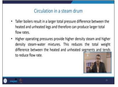
The Taylor boilers sometimes result in a large total pressure difference between the heated and unheated legs, which can produce a larger total flow rate. Sometimes higher operating pressure provides high-density steam and high-density steam-water mixture. This reduces the total weight difference between the heated and unheated segments and reduces the flow rate.
