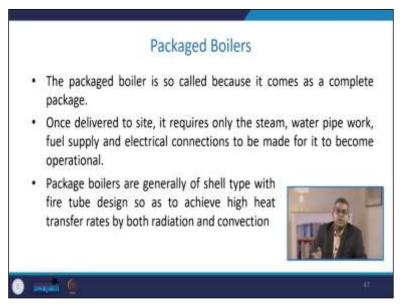
They are so-called package boiler because it comes as a complete package. So, once you deliver to the site, it requires only the steam. The water pipe piping network supply of fuel electrical connections, and you can start things. So, these boilers are generally of shell type with the fire tube design. So as to achieve a high heat transfer rate by both radiation and convection.
