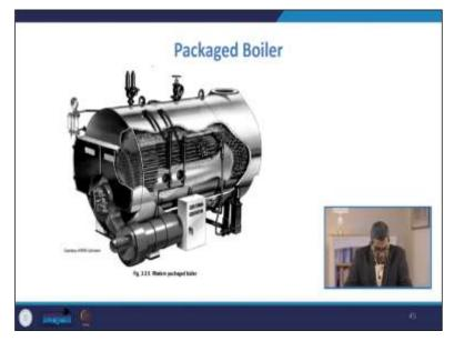
We are always looking for a compact assembly to minimize the space requirement in the modernday. So, the packaged boiler came into existence. You can see that everything is housed in this particular boiler. You can see the tubes, steam distribution wall manhole water level indicators firing media, etc. All these things are there.
