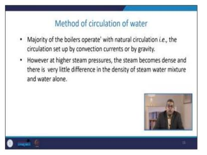
So, the majority of the boilers operate with the natural circulation, that is, the circulation set up by the convection current of gravity. Sometimes density difference is also attributed to this one. However, at higher steam pressure, the steam becomes dense, and there is very little difference in the density of the steam-water mixture and water alone.
