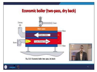
Another is the economic boiler two-pass dry back boiler. Dry back boiler we have already discussed in the previous slides. Now here you see that there is an externally fired burner and the chimney to discharge a flue gas. Here, to achieve maximum efficiency, the flue gases are passed in two passes for getting more and more efficiency.
