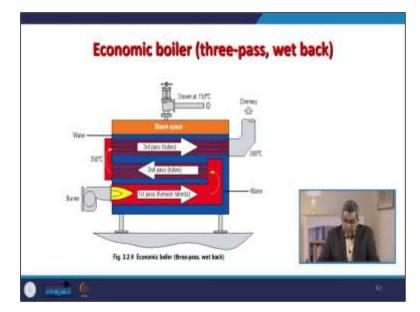
Similarly, we may have a wet back type of a three-pass system. Here you see the burners burner imparts the heat energy one pass, two passes, and three passes for the maximization of this thing, and you may get the steam at the desired temperature.
