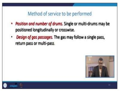
When we are talking about the classification, another classification is based on the position and number of drums. These may be either single or multi drum. This may be positioned longitudinally or crosswise. Another classification is steam; this steam is based on the design of gas passage. The gas may follow a single pass, return pass, or multi-pass.
