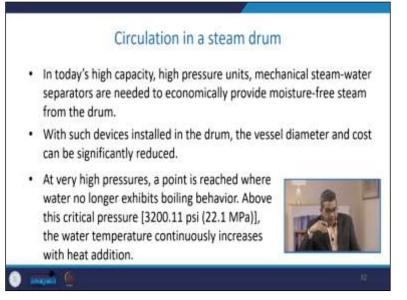
Now in today's high capacity, high-pressure units, mechanical steam-water separators are needed for the economical operation of any system where you require moisture-free steam from the drum. With such devices installed in the drum, the vessel diameter and the cost can be significantly reduced. So, a point is reached at a very high pressure where water no longer exhibits boiling behavior.
