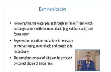
Following this, the water passes through an anion exchange resin which exchanges anions with the mineral acid and sometimes sulphuric acid, and it forms the water. Regeneration of cation and anion is necessary at intervals using mineral acid and caustic soda. Because all the active sites of these cations and anions may get blocked during the course of water treatment, it is necessary that
