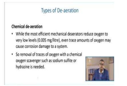
Chemical deaeration, the most efficient mechanical deaerators, reduces the oxygen to a very low level. Even trace amount of oxygen may cause corrosion damage to a system. Therefore, sometimes the chemical deaeration is also applied. So, to remove the traces of oxygen, this is being carried out with the help of chemical scavengers such as sodium sulfite or hydrogen.
