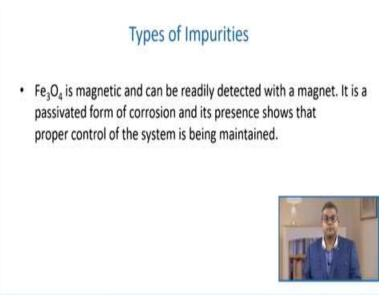
this magnetite it can be readily detected with magnet. it is passivated form of corrosion and its presence shows that proper control of the system is being maintained.
