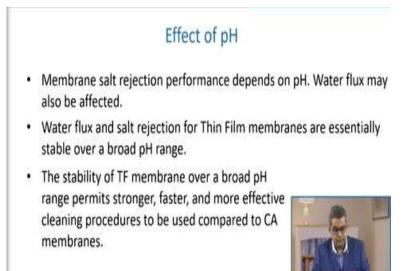
The membrane salt rejection performance depends on pH, and water flux may also be affected. So, thin-film membranes' water flux and salt rejection are essentially stable over a broad pH range. The stability of TF membrane over a broad pH range permits a stronger, faster, and more effective cleaning procedure to be used compared to cellulosic acetate membrane.
