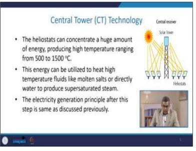
These heliostats can concentrate a large amount of energy-producing a high temperature ranging from say 500 degrees Celsius to 1500 degrees Celsius and sometimes even more.
