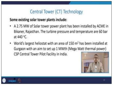
There are some existing solar tower plants, and this includes a 2.75 megawatt of solar tower power plant ACME has installed in Bikaner Rajasthan. The turbine pressure and the temperature are 60 bar at 440 degrees Celsius. The world's largest heliostat with an area of 150 square meters has been installed at Gurgaon to set up one megawatt or thermal power and is sometimes referred to as 1M WTH CSP central tower plant facility in India. (**Refer Slide Time: 07:28**)
