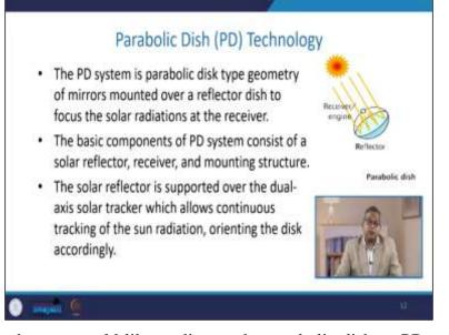
Another thing is that we would like to discuss the parabolic dish or PD technology. The parabolic dish system is parabolic disk-type geometry of mirrors mounted over a reflector dish to focus the solar radiation at the receiver. Here you see that the receiver engine and all these things are addressed to the receiver engine. The basic component of the parabolic dish system consists of a solar reflector and a receiver and mounting structure.
