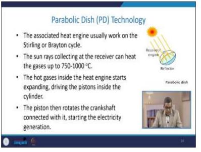
The associated heat engine it usually works on Sterling or Brighton cycle. The sun rays collecting at the receiver here you can see these can heat the gas up to 750 to 1000 degrees Celsius. The hot gases inside the heat engine have the tendency to expand, driving the piston inside the cylinder. The piston then rotates the crankshaft connecting with it and starting the generation of electricity.
