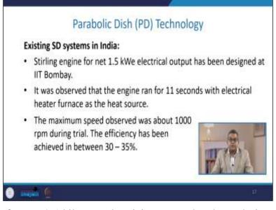
External engine for net 1.5-kilowatt electricity output has been designed at the Indian Institute of Technology, Bombay. It was observed that the engine ran for 11 seconds with an electrical heater furnace as the heat source. The maximum speed observed was about 1000 rpm during the trial run and have achieved an efficiency between 30 to 35%.
