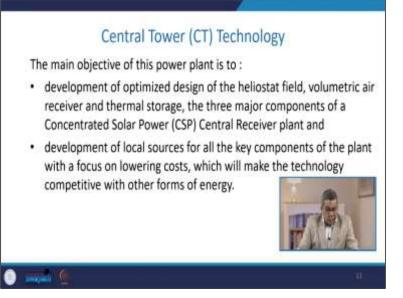
This power plant's main objective is to develop the optimized design of the heliostate field volumetric air receiver and thermal storage and three major components of concentrated solar power that is CSP the center is receiver plant. Another objective is to develop or development of local sources for all the key components of the plant with a focus on lowering costs which will make the technology competitive with other forms of energy.
