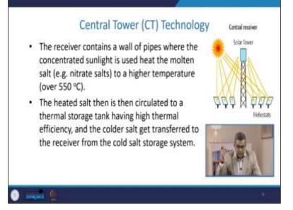
The receiver contains a wall of pipes where the concentrated sunlight is used to heat the molten salt, sometimes nitrate salts, to a higher temperature like 550 degrees Celsius or sometimes more. This heated salt is then circulated to a thermal storage tank with high thermal efficiency, and the colder salt gets transferred to the receiver from the cold salt storage system.
