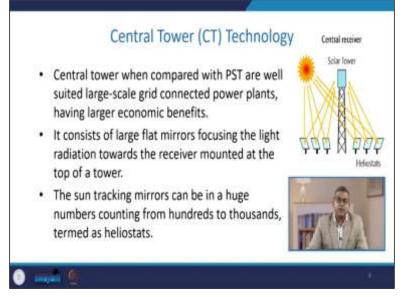
It consists of large flat mirrors like this here, you are having these large flat mirrors connected with the heliostats. These mirrors focus the light the radiation towards the receiver. This is a central receiver mounted at the top of a tower. These sun-tracking mirrors can be in a huge number counting from 100 to 1000, termed heliostats.
