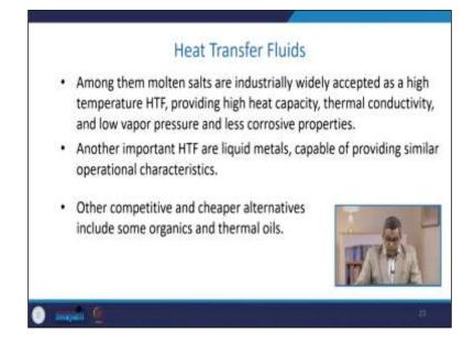
Another important heat transfer fluid is the liquid metals capable of providing similar operational characteristics, which we discussed for the molten salts. Other competitive and cheaper alternatives include some organic and thermal oils and organic, sometimes synthetic organic segments. In the CSP section, we have already discussed various things related to these heat transfer fluids. Usually, the higher efficiency is obtained at higher temperature operation.
