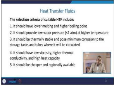
One criterion is that it should have a lower melting and a higher boiling point. It should provide low vapor pressure maybe sometimes less than one atmosphere at a higher temperature it should be thermally stable and pose minimum corrosion to the storage tank and tubes where it is it will be circulated it should have a low viscosity and higher thermal conductivity and higher heat capacity.
