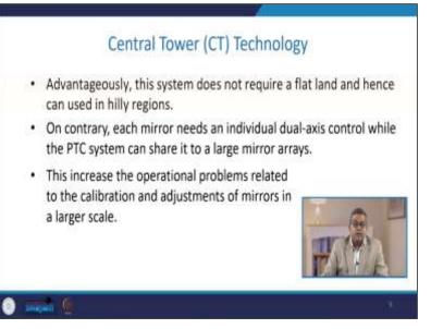
On the contrary, each mirror needs an individual dual access control while the PTC system can share it to a large mirror array. This increases the operational problem related to the calibration and adjustment of mirrors on a large spectrum or a large scale.
