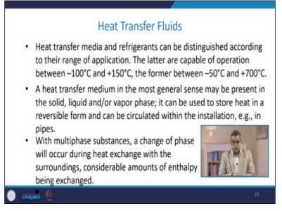
We have discussed a lot about solar energy and you see that whenever we are talking about solar energy, the integral component of this solar energy is the heat transfer fluid. As we previously discussed, heat transfer fluid offers a very good spectrum in all chemical engineering applications and especially when we look for heat transfer media, all these heat transfer fluids came into existence.
