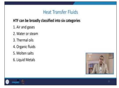
So, one category is air and gas. Second, maybe the water or steam then we have various thermal oils sometimes, the synthetic organic fluids or various organic fluids can be ac as a heat transfer fluid. Molten salts are a very good candidate of heat transfer fluid liquid metals are having wide range of heat transfer temperature differences. The molten salts are industrially wildly accepted as a heat high-temperature heat transfer fluid.
