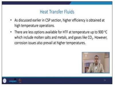
You can say the less options available for heat transfer fluid at a temperature up to 900 degree Celsius, which includes molten salt metal gases sometimes like carbon dioxide, etc. But when we go for a higher temperature the issue pertaining to the corrosion it also prevails. So, all these things while designing, selecting, and developing any kind of system must be addressed.
