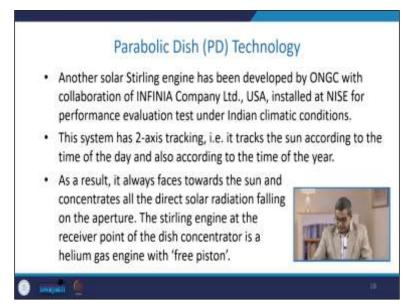
Another solar studying engine has been developed by ONGC in collaboration with Infinia Company, USA, and installed at nice and I see for the performance evaluation test under the Indian climatic condition. This system has 2x axis tracking, and that is, it tracks the sun according to the time of the day and also according to the time of the year. As a result it always faces toward the sun and concentrates all the direct solar radiation falling on that particular aperture.
