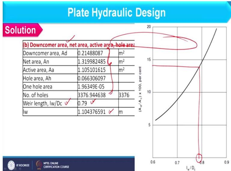
So, part B is we have to find out different areas and it will also depend on the column diameter. So, accordingly you can calculate this. Details of all these we have already discussed in 11th week. So, you can refer I am showing the values of this example here. So, as far as this weir length is concerned this is corresponding to 14% column area and that we can see from this graph.
