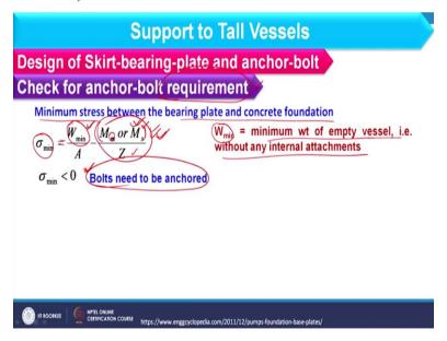
So, now we will focus on the anchor bolt and for that first of all we have to check whether anchor bolt is required or not. So, first of all let us see what is anchor bolt? Anchor bolt is basically the bolt which is attach with the concrete foundation. It means some part of the bolt
