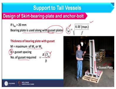
Now here we should check the thickness of bearing plate if thickness of bearing plate is more than 20 mm so what we have to do? In that case we should consider bearing plate along with the gusset plates. So, bearing plate you know if I consider this support so this is attach with this plate and this plate is basically called as the bearing plate. And we can put a metal plate in a triangular shape with right angle.
