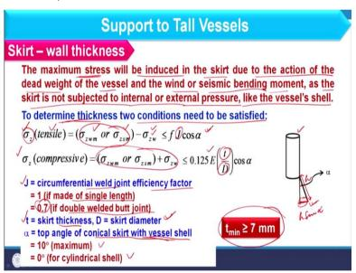
So, the maximum stress will be induced in the skirt due to action of dead weight of the vessel and wind or seismic bending moment as the skirt is not subjected to internal or external pressure like the vessel shell. So, if you recall the last lecture where we have discussed the resultant longitudinal stresses there we consider stresses generated due to dead load, due to operating pressure and due to wind load or seismic load.
