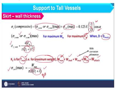
So, this is the expression we can have maximum compressive stress when this would be maximum and this would be maximum and that should be equal to 0.125 E t / D into cos alpha. So, you can understand that when compressive stress will be maximum if this is the support and I am having shell over here. So, whatever the maximum possible load will fall on this support compressive stress in this support would be maximum.
