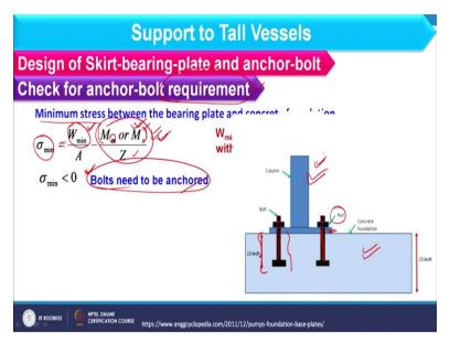
In that case let us see what is anchored bolt? If you consider this I am having the bolt and maximum part of this bolt is inside this concrete foundation and we can have some upper section also where this bearing plate is attach with this nut and here I am having the column with the support. So, we can understand that anchor bolts are required to remove or to avoid falling of the column or to avoid overturning of the column.
