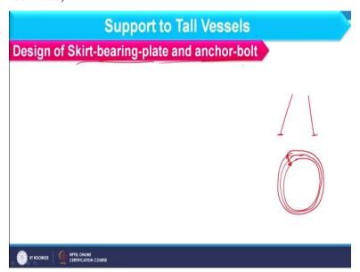
Now, we will consider few more parts as far as support of the tall vessel is considered. So, here we are considering design of skirt bearing plate and anchor bolt. So, what is bearing plate? When I consider shell like this at the bottom it is basically attach with the ring that is basically the metal ring. If you see the top view of this is basically the metal ring and shell is welded at the center of it or at one edge of it.
