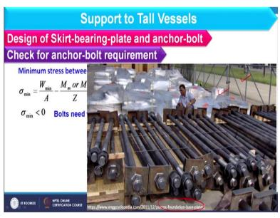
So, you can see the anchor bolt and size of these in this image detail you can find over here.
