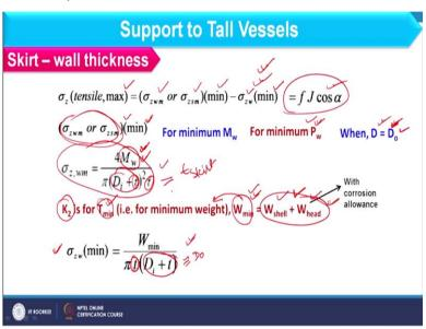
So, let us start the skirt wall thickness calculation. First of all, I am considering tensile stress so this is the expression. Now here you should understand the fact that so if I am focusing either on tensile stress or compressive stress I am basically considering the extreme condition. So, when that tensile stress will be maximum if I am having this shell right and column is available over it.
