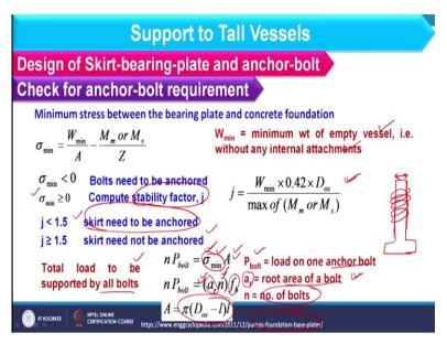
Further, if sigma minimum is greater than or equal to 0 in that case we should consider the stability factor j and j we can calculate by this expression. If j is less than 1.5 it means anchoring is required if j is more than or equal to 1.5 anchoring is not required. So, in this way you can check whether anchor bolts are required or not. Now, once it is required you have to calculate number of bolts as whatever total load is available that should be supported by all bolts.
