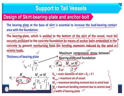
So, the bearing plate at the base of the skirt is essential to increase the load bearing contact area with the foundation because when you attach the skirt with the foundation or support with the foundation you are basically attach support with the bearing plate and then that bearing plate is attach with the foundation. So, bearing plate design is very important as far as support design is concerned.
