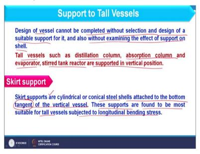
So, when we consider design of the vessel that cannot be completed without selection and design of the suitable support for it and also without examining the effect of support on the shell. So, in this way design of support is also as important as design of tall vessel or design of vessel. So, tall vessels when we consider these are basically distillation column, absorption column and evaporator, stirred tank reactor and these are supported in vertical position.
