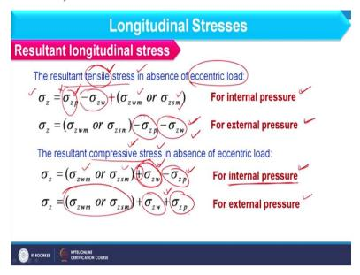
So, first of all I am considering resulting tensile stress and in this I am not accounting eccentric load. So, in this case we have sigma z as the resultant tensile stress and this is the expression and this expression is valid for internal pressure. So, if I am considering tensile stress which is generated in the shell it means it will try to expand. So, if I am having internal pressure in that case what will happen?
