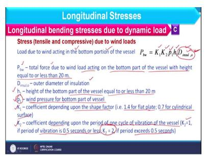
So, the load due to wind acting in the bottom portion of the vessel can be given by this expression that is P b w = K 1 K 2 p 1 h 1 and D insulation outer because when the wind will be there it will affect the outer most layer of the vessel. So, at that side usually we have insulation. So, as far as P b w is concerned this is the total force due to wind load acting on bottom part of the vessel with height equal to or less than 20 meter.
