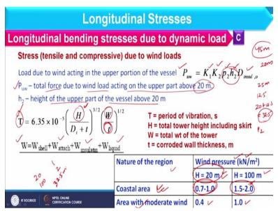
So, in this way we can count the load at bottom part of the vessel and now we will discuss load at upper part of the vessel. So, this can be considered as P u w K 1 K 2 p 2 h 2 D insulation outer. So, expression is same only p 2 h 2 will differ. So P u w is the total force due to wind load acting on upper part and that should be beyond 20 meter, h 2 is the height of the upper part of the vessel above 20 meter.
