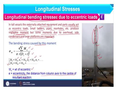
So, we consider that as eccentric load and because of that bending stress is generated in the shell. So, in the tall vessel externally attached equipment and parts usually act as eccentric load, small ladder pipes, manhole etcetera produce negligible moment, but some moment due to overhead, side condenser and large platforms are important. So, usually we neglect this part that is stress generated due to eccentric load.
