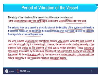
And now we will discuss few points about period of vibration of the vessel. So, usually period of vibration we can consider in two way. First is the vibration induced by the earthquake and second vibration induced by the wind. The seismic force on the vessel is also the function of the flexibility of the system and therefore it become necessary to determine the natural frequency of the vessel in order to calculate the magnitude of earthquake force.
