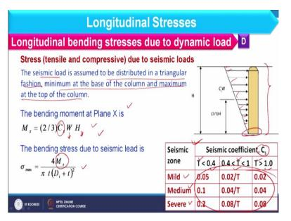
Seismic load is assumed to be distributed in triangular fashion minimum at the base of the column and maximum at the top of the column. So, if we consider the seismic load it means when earthquake will be there it effect will be less at the bottom. However, it will keep on increasing at the top. So, in this way we can consider the seismic load which is moving in triangular manner from bottom to top.
