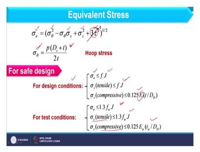
So, as far as equivalent stress is concerned that can be given by this sigma e which will be equal to sigma theta square – sigma theta sigma z + sigma z +
