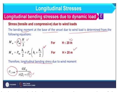
So, once I am having the wind loads at bottom and upper section of the column we can consider bending stresses. And to consider bending stress we will first focus on bending moment. So, the bending moment at the base of the vessel due to wind load is determined using this equation where H is less than or equal to 20 meter and therefore here we have counted P b w.
