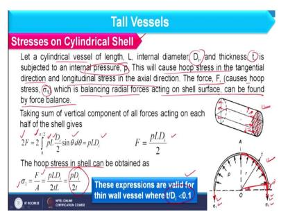
And these we consider as the stresses on the cylindrical shell. So, here we are considering a cylindrical vessel of length L with internal dia D i and the thickness t and it is subjected to pressure p. This will cause hoop stress in tangential direction and longitudinal stress in axial direction. So, if I am having this vessel which is basically the cylindrical in shape and this section is covered.
