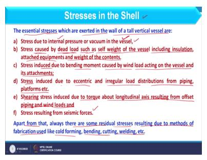
So, let us see that. So, as far as different stresses in shell is concerned we are going to discuss the essential stresses which are exerted in the wall of the tall vessel. So, first of all the stress due to internal pressure or vacuum in the vessel. So, when we consider that internal pressure and when we consider that external pressure is working. Internal pressure and external pressure vessels are defined as wherever we are having large pressure.
