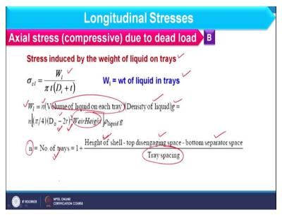
Next, we have stress induced by weight of the liquid on the tray if I am considering the tray column. So, in this case this is the stress W 1 / pi t D i + t and W I is the weight of liquid over the tray. And how we can calculate W I that should be equal to n volume of the liquid on each tray into density of the liquid into g. Further, n is the number of tray we can see how it will be calculated pi / 4 D 0 square -2 t square.
