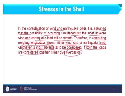
So, further we can see that in the consideration of wind and earthquake loads it is assumed that the possibility of occurring simultaneously the most adverse wind and earthquake load will be remote. And therefore in computing the resulting longitudinal stress either wind load or earthquake load whichever is most adverse is to be considered. So, this point we should consider while designing if both loads we consider we find that it is over design.
