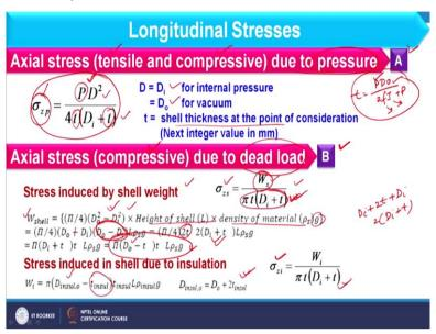
So, first of all we will consider the axial stress that is basically tensile or compressive and that should be due to pressure when it will be internal pressure we can have tensile stress because it will try to expand it and when I am having external pressure it will try to compress it so compressive stress will work there. And that we are counting as A because this is the first factor.
