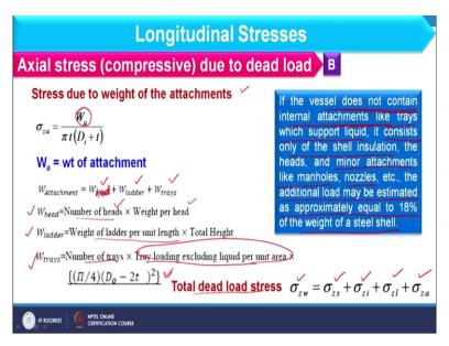
In dead load we have other factors such as stress due to weight of the attachment. So, this is basically total load of the attachment and it includes weight of head. So, this is basically head not the shell. Along with this, we have weight of ladder we can consider weight of trays because these are internal and external accessory which are attach to the equipment. So, weight of head is basically number of heads into weight per head.
