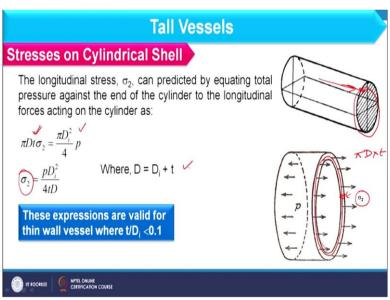
So, if we consider the longitudinal stress it will create sigma 2. So, that will be balanced by the forces which is generated in this shell. So, in that case pi D t into sigma 2. So, wherever this sigma 2 will act if I consider that mean dia so that pi D will be the periphery into t because t is the thickness of this wall. So, that will be the acting area into sigma 2 will be equal to the pressure which is generated over here and it will try to push it.
