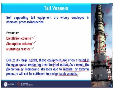
So, as far as this tall vessel is concerned this is basically the tall equipments and these type of vessels or tall equipment are basically self supporting. It means whatever conditions are generated in support of these vessels that is also a part of design because until unless support will not be strong vessel cannot remain stand. So, we have to consider all these factors such as the column itself as well as its support.
