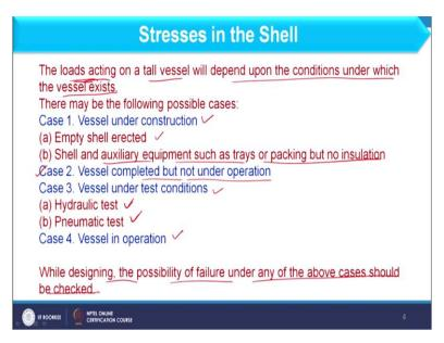
So, we can see that the loads acting on the tall vessel will depend upon the condition under which vessel exists and these conditions we can have with different cases. So, the case 1 is when vessel under construction it means empty shell erected where operation is not going on and no content is there. Shell and auxiliary equipment such as tray or packing, but no insulation.
