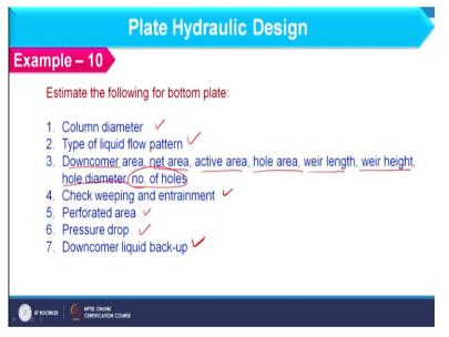
First of all we have to calculate column diameter then decide liquid flow pattern and then decide the plate layout that is downcomer area, net area, active area, hole area, weir length, weir height, hole diameter and number of holes. After that weeping and entrainment condition should be checked and maintained if these are not within the permissible range and next we have to find out perforated area then the pressure drop and then downcomer liquid backup.
