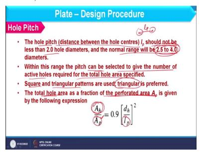
And next parameter in plate design is the hole pitch. So, let us see how to decide that and first of all we will focus on what is hole pitch that you understand it is the distance between hole centers like holes are there. So, this is basically the hole pitch which is denoted by small l into p. So, l p should not be less than 2 hole diameter and the normal range is 2.5 to 4 diameters and this condition we should also check in designing.
