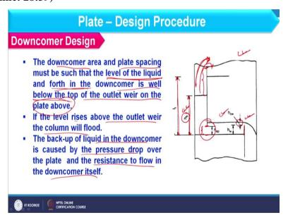
So, you can consider this schematic this Lt is basically the plate spacing and in this plate spacing this h b is the height of liquid available in downcomer section. So, if I have to design the downcomer properly this h b should be within the limit otherwise if this h b exceeds from
