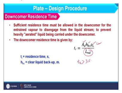
And finally we have downcomer residence time because sufficient residence time is required for downcomer for entrainment of vapour to disengage from the liquid stream and this is required to prevent the heavily aerated liquid which is being carried with the vapour in downcomer section. So, in this way we can find out the downcomer residence time and that can be calculated using this tr.
