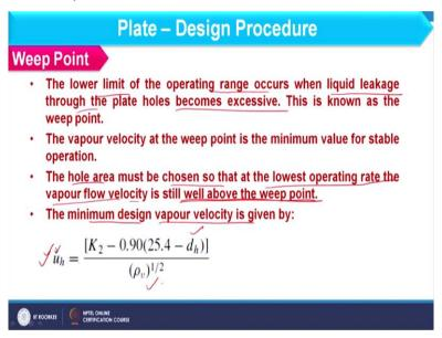
And further we will focus on weeping condition. So, as far as weeping condition is considered first of all we should understand what is the weep point? So, as far as weep is concerned I guess you understand that when liquid flow rate is very low it will start coming from the holes which are available for vapour to move up. So, in this way what we can say that if vapour velocity is low enough it will not able to hold the liquid over the plate.
