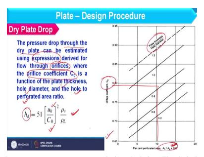
So, if you see what parameters we can account in ht calculation. First is h d which is the dry plate pressure drop second the static head and third is the residual loss h r. So, let us see first of all how to find out dry plate pressure drop that is h d. To find the h d pressure drop through the dry plate can be consider with the expression which is given over here. In this expression we basically consider that flow occurs through orifice.
