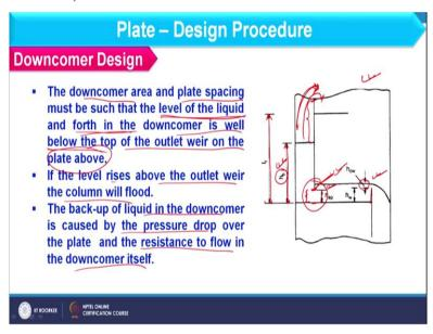
If you focus on this section so here I am having hap and this is available throughout the weir length or the chord of the weir. So, in that case we can consider the area as hap into L w which is the chord length as shown over here and how to decide hap that should be hw - 5 to 10 mm. So, for extreme condition we consider 10 mm deduction from h w. So, based on all these we can find h d c value and so h b value.
