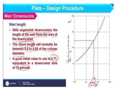
And now we will see how to find out weir length and what is weir length? If I am considering the cross sectional view of column then this is basically the weir length this we represent as small I w. So, that will depend on the downcomer area. So, with segmental downcomer the length of weir fixes the area of the downcomer. So, usually we consider this graph where A d / A c is there it means downcomer area percentage with respect to column area is given over here.
