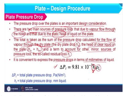
Now, once we have all dimensions of the plate we should consider plate pressure drop and as far as plate pressure drop is concerned this is basically an important design consideration. Here I am having two sources of pressure drop. First is due to vapour which flows through the holes and second is due to availability of the liquid on the plate which will cause static head.
