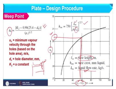
So that you can calculate from this graph here I am having K 2 on y axis on x axis we have hw + how. So, what is this hw this is nothing, but the weir height. What is how? This is basically the crest height over the weir. So, what is the crest height? Let us say if I am having this much height of the weir and liquid will move over this so whatever height of the liquid layer will make over the weir height that we consider as crest or we consider as crest or we consider that as weir crest.
