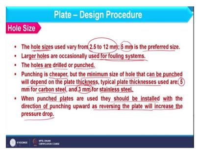
Next, we should consider the hole size and as far as complete range of hole sizes is concerned this varies from 2.5 mm to 12 mm. However, 5 mm is the preferable value. So, initial guess of hole size should be 5 mm and then depending upon the weeping condition you can vary this value in a given range. So, larger holes we usually consider when I am dealing with the fouling system with the obvious reasons.
