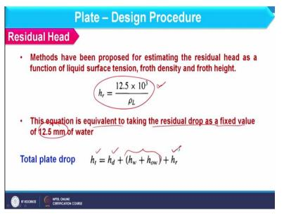
Next, is the residual head. Residual head is usually consider with the fixed value and that should be 12.5 into 10 is to the power 3 divided by rho L. So, this equation is equivalent to taking the residual drop as a fixed value of 12.5 mm of water. So, the total pressure drop is basically ht which is equal to h d h w + h o w that is static head and this is addition and here we have the residual loss.
