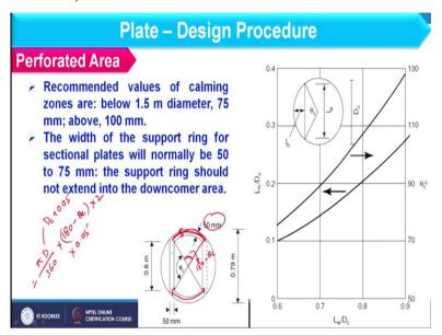
So, to decide the perforated area we have to deduct the area which are covered by the support ring as well as calming zone. So, first of all we will decide the thickness of calming zone as well as the support ring and as far as support ring is concerned it is only available where the plate is there. It means it is not extended to the downcomer section because if ring will be available and plate is not available because that is the empty section.
