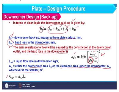
So, let us consider the downcomer design that we also call as the backup. So, in terms of clear liquid downcomer backup can be considered using this equation where h b should be equal to h + h + o + w + h that is the total pressure drop over the plate + h + d + c. So, let us see these parameters h t, h w and how we have already calculated h b here is basically the downcomer backup.
