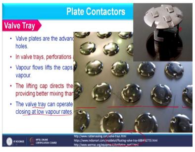
So, you can see the valve plate closely from this image and for details you can go through these links and as far as that cap is concerned it is basically looking like this. So, in this way we can have the valve tray.
