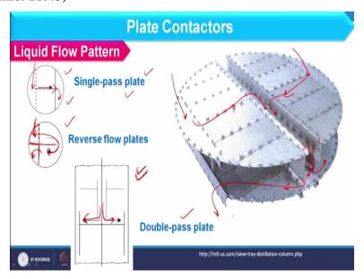
And here we have some flow patterns as well as liquid movement is concerned and here first of all we have single pass it means how the liquid movement occurs over the plate. So, if you consider here liquid is coming from the top moving over the plate only once and then coming down. So, this is basically single pass plate and in most of the cases such type of flow pattern is considered and second we have the reverse flow.
