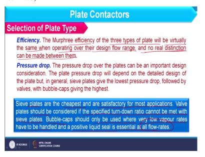
So, next point we have is the efficiency The Murphree efficiency of three types of plate will be virtually the same when operating over their design flow range and no real distinction can be made between them. So, as far as efficiency is concerned it is almost same for all and next we have pressure drop. As we have discuss that pressure drop is basically causing by the friction which is generated when movement of vapour as well as liquid is occurring.
