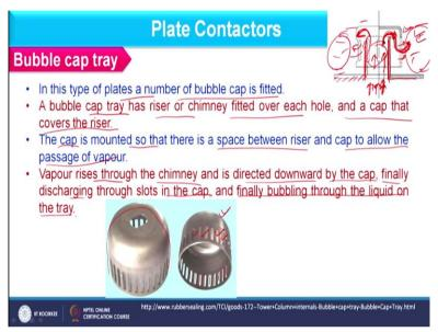
Now, let us focus on another plate and that is basically bubble cap tray. So, as far as bubble cap tray is concerned in this type plates are having number of bubbles cap. So, what is this bubble cap? It is basically the cap which has some sections where we can form the bubble. To give an example here we have the bubble cap. So, this is basically the cap complete cap is there where I am having these type of holes.
