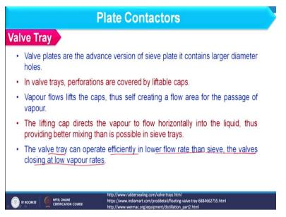
Further, valve tray can operate efficiently at low flow rate than sieve plate and as valves are closed at low vapour rates. So, weeping can be avoided.
