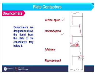
And now we will focus on the downcomer you can see different types of downcomers are there vertical apron, inclined apron like this and here we have inlet weir also like from apron liquid is coming down and then here we have some restrictions and after that the movement of the liquid over the plate has more turbulence. So, we can have better mixing over here and similarly I can have the recessed well as you can observe here.
