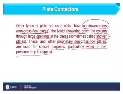
So, let us start with the sieve plate. However, when we focus on the plate apart from sieve plate, bubble cap tray as well as valve tray we have another type of trays also such as showers plates. So, these are basically plates which does not have any downcomer. So, non cross flow occurs over the plates. Liquid is basically showering down the column through large opening in the plate and therefore it is called as shower plates or we consider that as a shower plate also.
