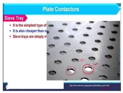
Further, this image you can see where you can find the holes closely. So, this is simple. The metal sheets were close so here we have the metal sheet where holes are available like this you can see and for details you can go through this link about the sieve plate. So, further let us consider few more points about sieve plate and this is basically in the sieve plate vapour passes straight upward through the liquid on the plate as we have discussed previously also.
