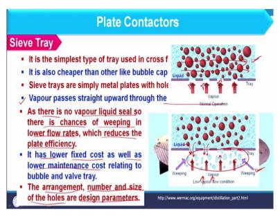
And that you can also imagine from this schematic like here I am having the vapour which is moving from downward and this is basically the normal operation where liquid is available and then whatever vapour is entering from the bottom it will be available in the form of droplets as you can see in this diagram. And further if weeping will occur then what will happen?
