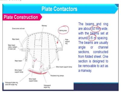
And here we have some plate constructions and we will quickly cover it. Here, you see when the liquid is coming over the plate it is basically the section where holes are not available so it is called as calming area and here we have the metal ring which we call as the support and over this support tray lies or tray sits. And when the size of the diameter is very large we prepare this plate in different sections.
