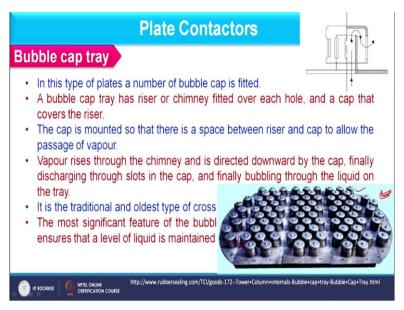
Now, if you see the most significant feature of bubble plate is that it uses the riser and that riser is basically stopping the liquid from coming to the plate through the hole to downward. So, that chimney as well as riser is working as the stopper for liquid to move downward and therefore weeping is not possible in these types of trays and when we consider very low liquid flow rate then also liquid is not able to move from the slots of the cap to the chimney and so through the hole.
