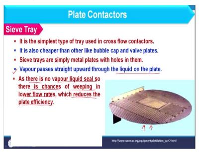
So, as far as sieve plate is concerned this is basically the simplest type of tray which we consider in cross flow contactors. And when you see the image of this it will be like this. So, it is basically the plate where simple holes are there and if you consider this section here solid plate is there no pores are available. So, this is the area where liquid is falling from upper plate and this is below the downcomer section.
