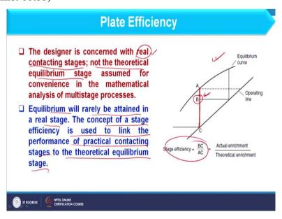
Now, as far as this plate efficiency is concerned why it is required? Because we do not reach up to the desired separation which should be reached in ideal condition. So, in that case if we consider this schematic there you see we can consider enrichment from C to B. However, I am suppose to consider the enrichment from C to A and that difference is basically considered in calculation and that is represented by stage efficiency.
