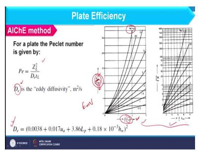
So, you can consider this Peclet number and that is basically Z L square / D e into t L and D e is basically the eddy diffusivity which counts the mixing over the plate and this is the empirical correlation to calculate eddy diffusivity. And once you have the Peclet number you can find out this m V / L E m v because E m v you can already calculate based on N L as well as N G value.
