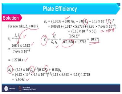
So, that we should avoid and therefore we will consider another value of Z c for further calculations and this value is 0.019. So, in that case we can calculate t L where Z c you can consider and Z L you can consider and L p and so t L you can obtain as 1.2718 seconds. So, considering all these values you can find N L because all these parameters you have already calculated and so N L can be obtained as 2.6642.
