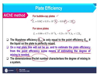
So, in that case we consider the bubble cap plate where Z c you can obtain by this expression where h w is the weir height Fv and L p all these we have already calculated and for sieve plate we can use this particular expression. What is this bubble cap, sieve plate and wall tray these trays we will consider when we will discuss the plate hydraulics. So, that will come in subsequent lectures.
