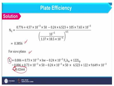
And so N G value you can obtain as 0.3856 and next we have to find out N L and for that I need Z c and for sieve plate because this plate is given in this problem you can find Z c value
