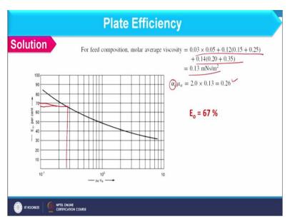
So, in this way you can find out the average molar viscosity of the liquid in feed and alpha a is already known to you. So, you can find out this factor which comes out as 0.26. So, if you see here I am having 1 and this is 2 so here I am having 0.26. So, the value you can obtain from here and that should be 67%. So, in this way you can simply calculate overall column efficiency.
