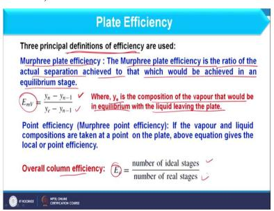
So, let us revise that and then we will discuss plate efficiency in detail. So, usually we have three principle definitions of the efficiency. The first one is the Murphree plate efficiency and this Murphree plate efficiency is the ratio of actual separation achieved to that would be achieved in equilibrium stage. So, that should be yn - yn - 1 divided by ye - yn - 1. So, in
