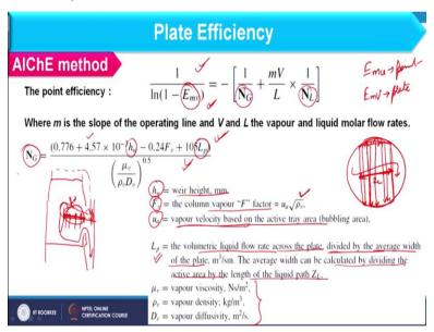
So, let us start this. As far as AIChE method is concerned, first of all we will consider point efficiency using AIChE method and then we will calculate the plate efficiency. So, let us see the expression of point efficiency first. So, here I am having the expression for point efficiency where E m v is the point efficiency. What is the difference in point efficiency and plate?
