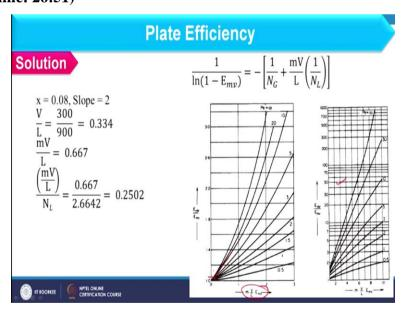
Here, I am having plate efficiency and this parameter I have to calculate first which I can obtain as 0.1974 and that value will lie somewhere here and Peclet number curve is here. So, the value will be very close to 1. So, if we will see E m v / E m v small the value should come as 1.08 that we can obtain by carefully seeing the graph. So, plate efficiency we can obtain as 31.9%. So, in this way we can solve the example.
