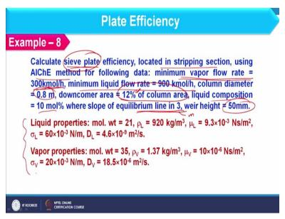
And now we will discuss this method based on example. So, here I am having example 8. In this example, we have been asked to calculate sieve plate efficiency. So, type of plate is fixed which is located in stripping section and this we have to carry out using AIChE method. Minimum vapour flow rate is 300 kilomole per hour, minimum liquid flow rate is 900 kilomole per hour, column diameter is given as 0.8 meter, downcomer area is 12% of column area.
