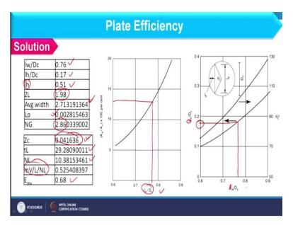
And here we have to find out first Z L. How I can find out Z L? I need to find out 1 h. So, if you consider the downcomer area is 12% of the column area. So, if I consider this graph here it is around 12% and corresponding to this I can find out 1 w / D c which should come as 0.76. So, 1 w / D c we can use in this graph where this is basically small I only and this is the small h only.
