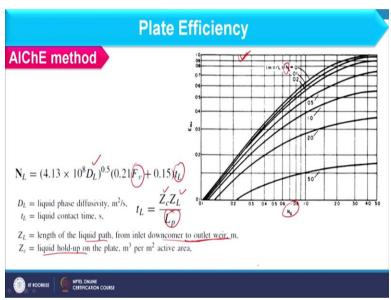
Instead of using that equation of E m v you can also use this graph, but in both cases we need N G as well as N L value. N G we have already calculated. This is the N L expression where F v we have already discussed in the last slide D L is the diffusivity of liquid and t L is the liquid contact time and that can be calculated by Z c into Z L / L p. So, Z L is the length of the liquid path from inlet downcomer to outlet weir that we already discussed in the last slide.
