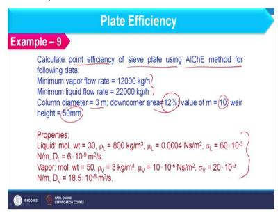
Now, quickly we will cover another example. Here, we have to calculate point efficiency for sieve plate considering AIChE method these are the flow rates of vapour and liquid, column diameter is given, downcomer area is given as 12%, value of m is given as 10, weir height is 50 and these are some of the properties.
