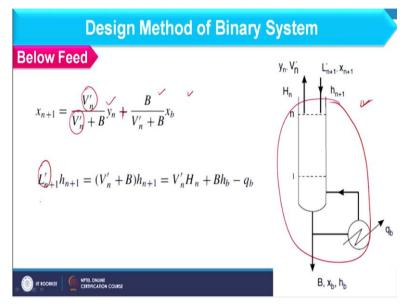
Now similarly we can find the balance at below feed and here we can make the balance and making the envelope like this. So, I am not going into detail of derivation of the equation. We can simply have the equation as x n + 1 which will be equal to V dash n / V dash n + B into y n and then plus and we can have B / V dash n + B into x b. So, you can see here we are representing the vapour flow rates as well as liquid flow rates with prime.
