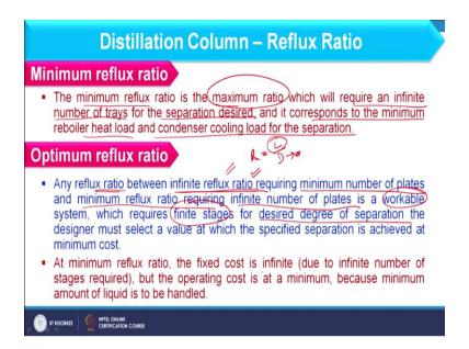
And now we have minimum reflux ratio if I am having total reflux we can consider minimum number of stages. Minimum reflux gives maximum number of stages. So, basically minimum reflux ratio we consider as the maximum ratio at which we require infinite number of trays for the given separation and it corresponds to the minimum reboiler heat load and condenser cooling load for the separation.
