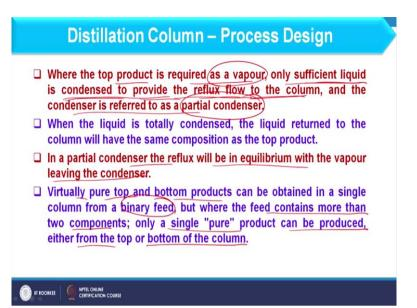
So, further in distillation column where the top product is required as vapour when I am considering the distillate at the top if that is required at the vapour only sufficient liquid is condensed to provide the reflux flow to the column and condenser is referred as the partial condenser and this point we have also discussed when we were discussing the topic of condensation and design of condensers.
