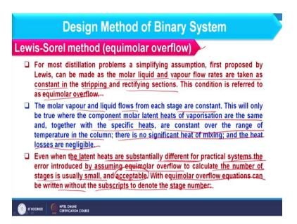
Now, further we can have some assumptions and based on that we will design the binary system. The assumption is like whatever molar flow rate we are considering either for liquid and vapour. So, these molar flow rate will be constant in each tray. So, throughout the distillation column these vapour flow rates as well as liquid flow rates will be constant. Like if I am considering L n or V n so that should be L and V throughout the distillation column.
