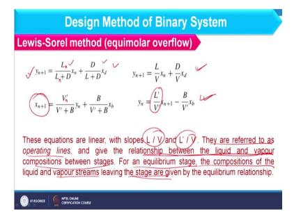
So, when I am assuming this we can represent the equations like y n + 1 should be equal to L / L + D into x n and additionally we further consider D / L + D x d. So, you can see we are not considering n over here like this. So, this should not be considered because equimolar overflow we have assumed. And when we resolve this equation we can obtain equation like this and when we consider this equation we can find revised equation as like this simply rearranging and considering the balances.
