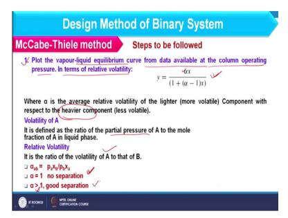
So, initially we have to plot the vapour liquid equilibrium curve from the data available at the column operating pressure and in terms of relative volatility and we can consider that equilibrium curve with this equation. So, where alpha is basically the relative volatility of lighter component and that relation we consider with respect to heavy component. So, you can see here I am having mol fraction in vapour that is y as well as x on x axis.
