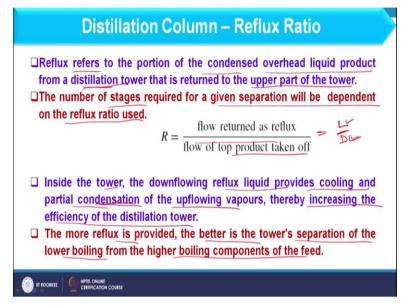
So this point we have already discussed that reflux refers to the portion of the condensed overhead liquid product which is coming to the distillation column and it is basically returning at upper part of the column. And the number of stages required for the given separation will depend on the reflux ratio. As we have variation in reflux ratio, we can consider different number of stages in plate column.
