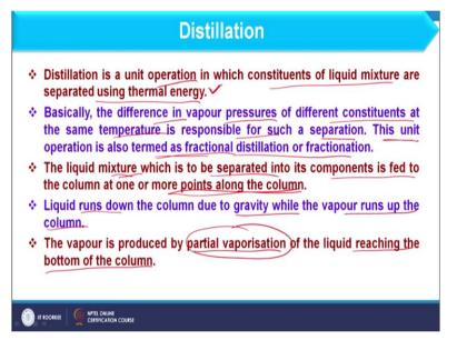
So, as far as distillation is concerned it is basically the unit operation in which constituents of the liquid mixture are separated using thermal energy and that thermal energy we usually provide in the reboiler. So, basically the difference in vapour pressures of different constituents at the same temperature is responsible for such separation. This unit operation is also termed as fractional distillation or fractionation.
