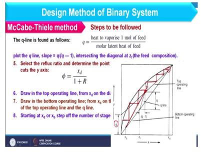
So, you can see this graph where I am having this phi value. So, this is basically the top operating value that is x d. So, from here to here you can draw the line wherever it will cut the q line from x b to that point we can draw the line and you can see from x d to x b we keep on steeping and in this way we can find the number of stages. So, in this way you can use McCabe Thiele method to find the number of stages for binary system.
