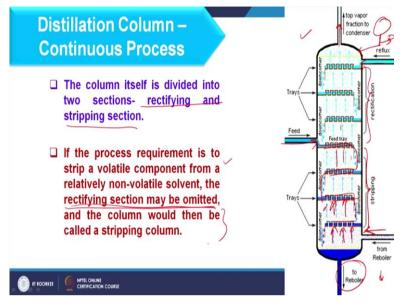
If you consider this schematic here we have the feed which is entering into the distillation column and on each tray mass transfer occurs between liquid and vapour. So, liquid moves in this way and vapour moves from the middle you can see here as you can see the arrows are shown upward. So, the section below the feed tray we consider that as a stripping section and this is rectifying section.
