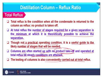
The first one is the total reflux. So, when I am considering the total reflux it means all condensate is returning back to the column. And in that case we are not considering any product which is exiting the distillation column from top. So, distillate will be zero so R value should be infinite. So, in that case distillate will be zero. So, total vapour which is exiting it is converted into condensate and that is returning back to the column.
