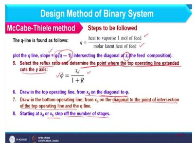
And this q line can be considered as q should be equal to heat to vapourize one mol of feed divided by molar latent heat of feed. So, we can plot the q line with the slope which is equal to q / q - 1 and intersecting the diagonal at Z f which is basically the feed composition. So, if you consider this graph here I am having the same curve that is the equilibrium curve like this and here I am having the feed condition and from this I can draw the q line.
