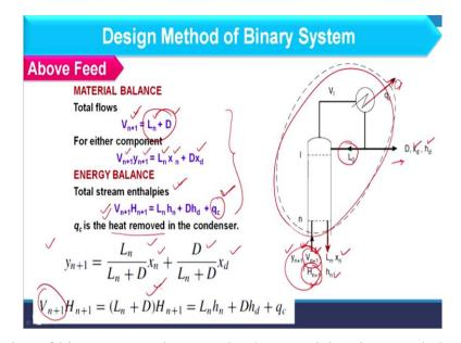
So, to start design of binary system let us make the material and energy balance. So, we are considering above feed system so here you can consider the distillate and this is basically the reflux and if we consider material and energy balance we usually make the envelope and in this envelope whatever stream is entering is that V n + 1 that is basically the vapour stream which is exiting n + 1th tray.
