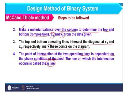
And further second step is to make the material balance over the column to determine top and bottom composition that is x d as well as x b from the given data. The top and bottom operating line intersect the diagonal at x d and x b respectively and we have to mark these points on the diagram. We will see all these points in the diagram also in the next slide. The point of intersection of two operating lines is dependent on the phase condition of the feed and so we consider the q line.
