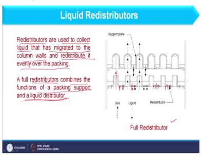
So, in this way redistributors are used and these are basically considered to collect the liquid that has migrated to the column walls and redistribute it evenly over the packing. So, it basically collects a liquid and redistribute it again. A full redistributors combines the functions of a packing support and liquid distributor. So, you can consider here we have the full redistributor and here we have the nozzle for the proper distribution.
