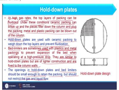
So, next we should consider the hold down plates. Now, what is this hold down plate? So, if we consider the packing then what will happen because gas is continuously coming from the bottom. So, what will happen it sometimes carries the packing with it if packing weight is less if we compare the metal as well as ceramic the ceramic packing is having lesser weight
