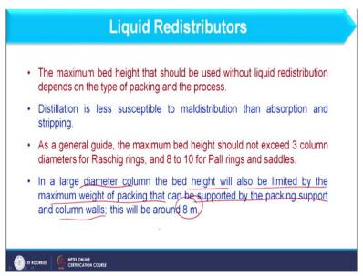
And now we have few more points about the liquid redistributor. In this the maximum bed height that should be used without liquid redistributor depends on the type of packing and the
