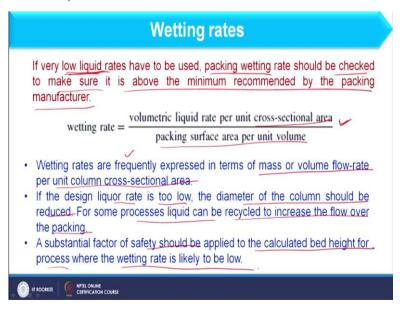
So, what is that wetted rates? This is basically the volumetric liquid rate per unit cross sectional area divide by the packing surface area per unit volume. So, if we consider this it should come out as the unit length per second. So, if we consider low liquid rate and that is basically very low liquid rate packing wetting rate should be checked to make sure that it is above the minimum recommended by the packing manufacturer.
