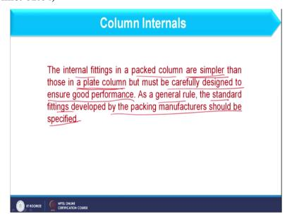
So, as far as internal fittings in the packed column are considered these are simpler in comparison to that we consider in plate column and it must be carefully designed to ensure good performance. So, what these internals are? These internals are basically liquid and gas distributor, packing support and we can have hole plates also. So, all these we consider apart from packing in the column and that we consider as the column internals.
