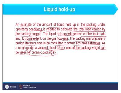
So, what it is an estimate of the amount of liquid held up in the packing under operating conditions is needed to calculate total load carried by the packing support. So, as we have discussed previously that packing support not only support the packing not only bear the weight of the packing, but also bear the weight of the liquid also. So, the liquid hold up will depend on the liquid flow rate and to some extent on the gas flow rate.
