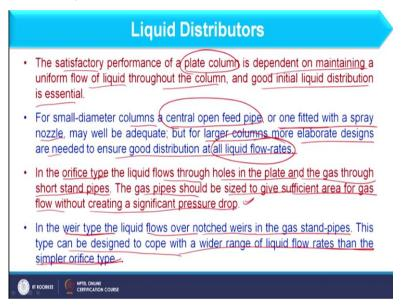
So, the satisfactory performance of the packed column is dependent on the maintaining a uniform flow of the liquid throughout the column and good initial liquid distribution is essential. In this we can consider a center open feed pipe or one fitted with the spray nozzle and through these nozzles liquid can be properly distributed in the packing when the column diameter is small.
