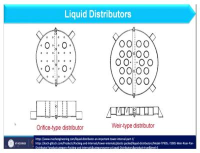
So, let us see here this is basically orifice type distributor where liquid will pass through from this small holes. However, these pipes are basically used for gas to move. So, these pipes are having some height however these holes are simply available on the plate and this is basically the weir type distributor where whatever pipes are available for gas it has a notch.
