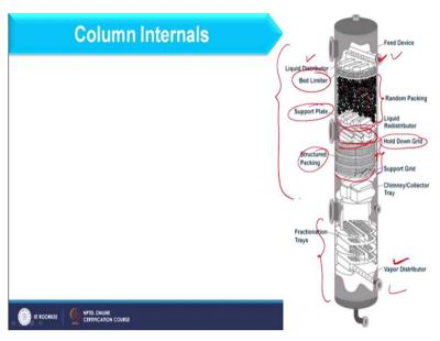
And if you see here I am having the top of the column and bottom of the column is shown over here. So, here we have vapour distributor and at top we have liquid distributor and then we put a bed limiter which does not allow the bed to expand and after that we can put the random packing and below the random packing support plate should be used. And if you see here I am having the liquid distributor up to here the liquid will be distributed and after that packing is not available.
