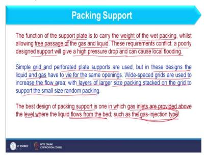
So, packing support should be properly selected and for that we can have some points as the function of the support plate is to carry the weight of the wet packing while allowing free passage of gas as well as liquid. So, as far as this packing support is concerned it should hold the liquid along with the weight of the packing. So, we can consider that as wet packing. So, these requirements conflict and poorly designed support will give a high pressure drop.
