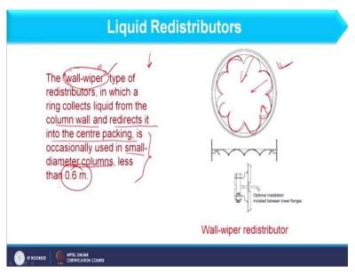
And now we have another type of liquid redistributor here we have wall wiper type redistributor as the name says it is wall wiper it means it is attached to the wall of the column and wipe the liquid inside the column. So, in which ring collects the liquid from the column wall and redirects it into the center packing. If you consider this schematic at the periphery we have this type of arrangement which we consider as the ring which collects the liquid and directs it towards the center.
