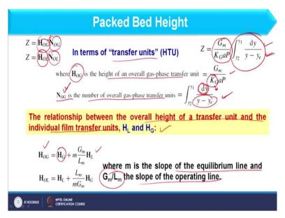
Now, we will relate this with the individual values. So, the relationship between overall height of transfer unit and individual film transfer unit that is H L and H G that relation is basically H O G = H G + m G m / L m into H L. So, to find out H O G we need to find out H G and H L and for that we should know m G m / L m. So, what is m? M is basically the slope of equilibrium line at a particular concentration at G m / G l is the slope of the operating line.
