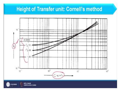
And now we have the graph of phi h. So that can be calculated based on Lw star and this value you can obtain once you know the column diameter. So, depending upon the size of Berl saddle you can find the value of this parameter. So, in this way you can obtain K 3, phi h and psi h value, but that require again a parameter that we consider as the percentage flooding.
