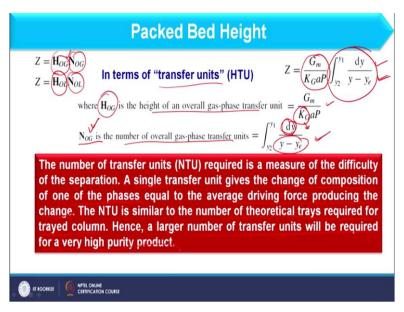
Next, I am having N O G which is basically the number of overall gas phase transfer unit and that can be equal to this term. So, it is showing over here also. So, if you see here we have integration from y 2 to y 1 and that will be d v divided by y minus y e. So, in this way we will integrate and find the N O G value. So, how we can define this number of transfer unit that we consider as NTU.
