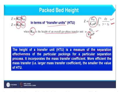
So, let us start the calculation of bed height and here we will focus on calculation of bed height based on transfer units that we consider as HTU. So, here you see we have this expression which we have discussed previously also. And this equation we can represent in terms of transfer unit as Z is equal to H O G and N O G. So, as far as these H O G and N O G values are concerned that value we can extract from this expression only.
