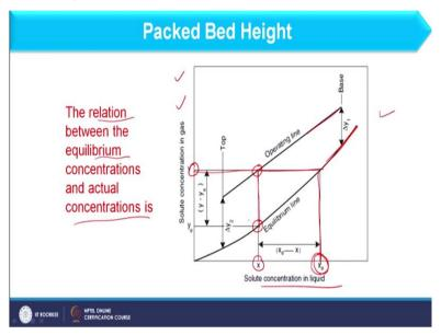
Now, as far as different in concentration in gas phase as well as liquid phase is concerned for that we can consider this graph and this graph is basically showing the relation between the equilibrium concentration and actual concentration. So, when you focus on this graph this is basically solute concentration in gas phase on y axis and here I am having solute concentration in liquid phase on x axis.
