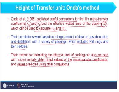
So Onda has given the correlation for the film mass transfer coefficient that is k G as well as k L. And effective wetted area of the packing that is aw which can be used to calculate H G as well as H L and their correlation are based on large amount of data on gas absorption and distillation with variety of packing which include Pall rings as well as Berl saddle. However, Cornell's correlation is basically used for Berl saddles.
