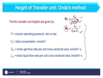
So, once you have the value of mass transfer coefficient in gas and liquid phase Onda's method relates it with the H G and H L value as H G is basically G m / k G a w P. This is the previous expression when we have considered the Z expression however that is based on effective area as well as gas phase mass transfer coefficient and similarly I am having H L value that can be given as L m / k L a w C t.
