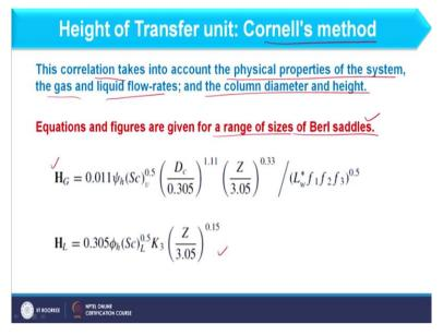
So, first let us focus on Cornells's method. So, as far as this method is concerned this correlation that is proposed by the Cornell's it considers the physical properties of the system, the gas and liquid flow rates and the column diameter and height. So, whatever correlations are given for H G and H L value these are basically for Berl Saddle packing. So, we can consider for a range of sizes of Berl saddle.
