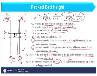
So, to calculate the bed height we should consider schematic of the packed column as it is shown here. So, if you consider this packed column this is basically the packing and here we have consider some section along the length and that should be Y + Y d and Y when I am considering the concentration in gas phase. And similarly I am having X + d X and X. So, usually we have counter current movement of liquid and gas.
