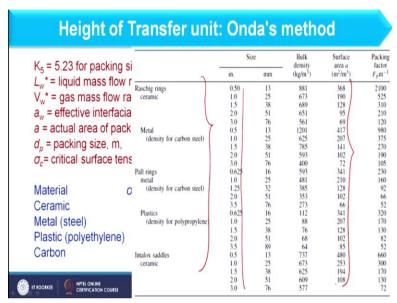
And here I am having the complete table of the packing and you see depending upon the size that is basically d p value you can find out area from here. So, in this way you can consider the parameters which are related to the Onda's method.
