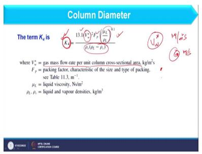
Now see how to calculate the column diameter. To find out that we will consider K 4 because K 4 is the parameter which is corresponding to the flooding condition. So, this K 4 is the parameter when we can obtain it at desired pressure drop. So, the expression is like 13.1 V w star power 2 F p and this is the and this is the physical property and here also we have the physical property of liquid as well as gases.
