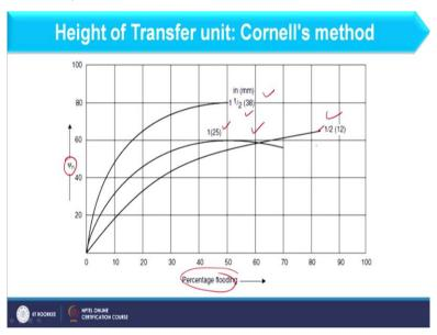
Similarly, you can obtain phi h value depending upon the percentage flooding and different types of packings. These packing are basically Berl saddle and having different sizes. So, in this way you can use this graph.
