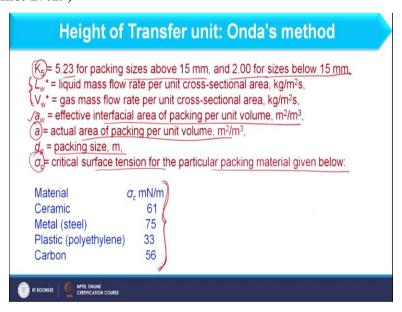
Now as far as parameters are concerned here I have to consider K 5 you can see here I am having the value of K 5. So, its value is equal to 5.23 for packing size above 15 mm and 2 for the packing size below 15 mm, L w star and V w star we have also discussed in Cornell's
