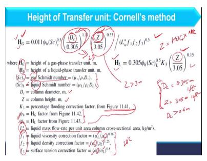
So, here again I am having the equation of H G as well as H L. So, you can consider different parameters as H G and H L are known to you so that is not the point to discuss. S c v and S c L are basically Schmidt number corresponding to gas and liquid and you can obtain from this expressions. D c is the column diameter Z is the column height. And K 3 is basically percent flooding correction factor and that you can obtain from figure 11.41.
