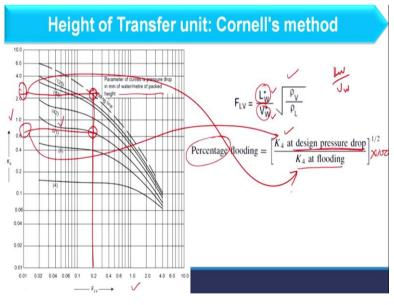
So, percentage flooding you can obtain by this expression and this graph. So, here I am having percentage flooding as we can find out K 4 parameter at design pressure drop and K 4 at flooding condition power 0.5 into 100 because this is basically the percentage flooding. So, if you consider this here on y axis I am having K 4 value and on x axis we have FLV value and FLV value you can obtain from this.
