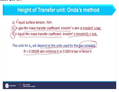
And further we have some points about the Onda's method as sigma L is given as the liquid surface tension. K G and k L are gas film mass transfer coefficient and liquid film mass
