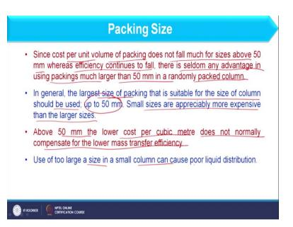
Further, since cost per unit volume of the packing does not fall much for sizes above 50 mm whereas efficiency continues to fall. There is seldom any advantage in using packing much larger than 50 mm in randomly packed column. So, here you should have the guideline that packing should be less than 50 mm because above that cost will not affect much however efficiency of the column reduces significantly.
