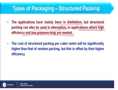
Further, as far as application of structured packing is concerned these are mainly used in distillation. However, structured packing can also be used in absorption in applications where high efficiency and low pressure drop are required. So, in this way you can select the proper
