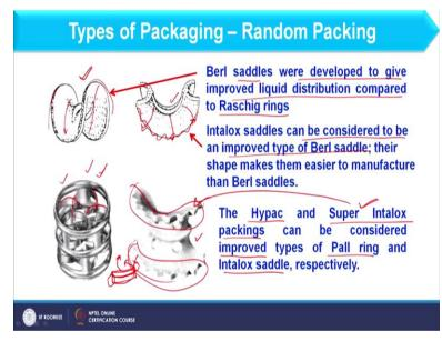
And next we have Berl saddle. So, this type of packing that is Berl saddles were developed to give improved liquid distribution compared to Raschig rings. So, you can consider this is basically the Berl saddle and how it is prepared when I am having the circular metal sheet and from two end we will fold like this and from two end we will fold like this. So, if you make flat of it is basically circular shape.
