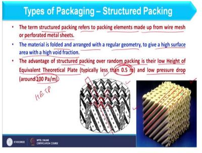
And now we have another class of the packing that is the structured packing. So, that you can understand structured packing are basically when we arrange the packing in a proper or in a definite manner. So, what these packings are? The term structured packing refers to packing elements made up from wire mesh or the perforated metal sheets. As you can see here we can have proper arrangement of the wire as well as metal sheet.
