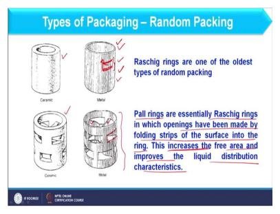
Let us see what are the different types of random packings available. The very common is basically the Raschig rings. So, as far as this type of packing is concerned it is the oldest type of random packing and if you see its structure it is basically like small cylinder and here we have the Raschig rings of the metal and here it is consider with ceramic. So, you can say ceramic has large thickness in comparison to metal to sustain same pressure conditions.
