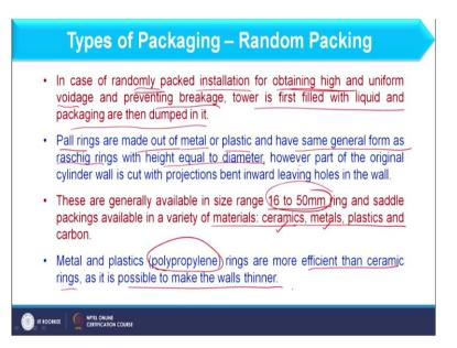
Now, let us focus on some points about the random packing such as in case of randomly packed installation for obtaining high and uniform voidage and preventing breakage tower is first filled with the liquid and packing are then dumped in. So, we can simply put the packing not in an empty column, but we can first fill the column through the water and then we put the packing into this.
