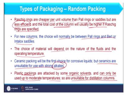
So, Raschig rings are cheaper per unit volume in comparison to Pall rings or saddle, but these are less efficient. So, if I am having the less cost that can be offset by less efficiency also because it does not have proper distribution of liquid inside the ring. It has a simple cylindrical wall and over that whatever interaction of liquid and gas occurs that can be considered.
