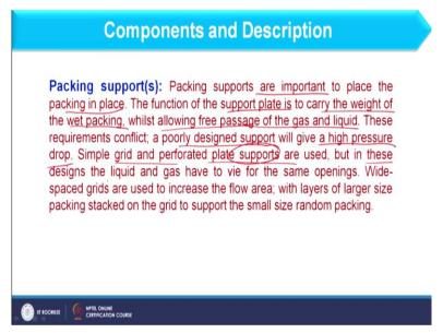
And next we have the packing support. So as far as this support is concerned it is important to place the packing in place otherwise packing will not be proper. So, the function of the support plate is to carry the weight of wet packing while allowing free passage of gas as well as liquid because when we consider the packing support its role is basically to hold all weight.
