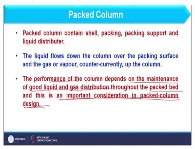
So, as far as packed column is concerned the complete assembly of packed column includes the shell which is basically the cylindrical section where packing is done and along with shell we have some other accessory such as packing which is basically filled in the shell and if packing is there we provide that with packing support as well as liquid distributor. So, these are some of the accessories which are used in packed column.
