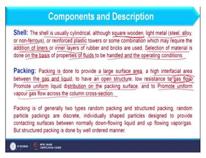
So, first of all we will focus on the shell so if you consider the shell this is basically cylindrical. However, sometimes we consider square wooden shell also. It is basically made with the light metal such as steel, alloy or nonferrous material or it can be reinforced with the plastic and which has some addition of liners or we can say the inner layer of rubber or brick. So, in that way we can mix different material and make the reinforced shell.
