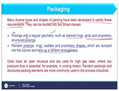
And we have some more points about this like as far as packing is concerned many diverse types and shapes of the packing have been developed to satisfy these requirements which we have just discussed. So, we can broadly classify the packing as packing with the regular geometry here you can consider packing such as stacked rings, grids and proprietary structured packing.
