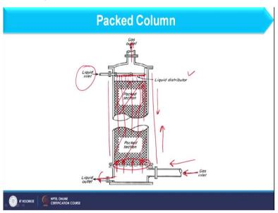
And here I am having the packed column schematic. So, if you see this is basically the shell and that shell has complete packing. So, this we consider as the packed section and as far as liquid movement is concerned we have already discussed that it enters from the top and moves downward and similarly gas enters from the bottom and moves upward. So, liquid enters from here and then it is passing through the distributor where uniformly it is falling over the packing.
