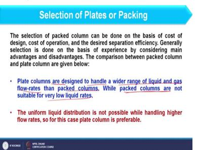
So, as far as selection of packed column is concerned it is basically based on cost of the design and cost of the operation. And after that we consider the separation efficiency which is basically the desired separation efficiency and to choose the proper column we first should consider the advantages and disadvantages of each type. So, when I focus on a plate column these are designed to handle a wide range of liquid and gas flow rates than the packed column.
