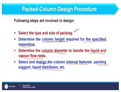
And now we will focus on packed column design procedure. So, the steps are first of all we will choose proper packing, its size and after that we will calculate the column height which is required for specified separation and further we can calculate the column diameter to handle the liquid and vapour flow rates. So, all these points we will discuss while considering detailed packed column design.
