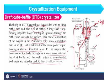
Now, we have draft tube baffle crystallizer. In this case this is the schematic you see here we have this structure that is nothing, but the tube and this we call as the draft tube and as far as baffle are concerned this is basically the baffle. So, in this case what will happen heated feed enters the center of the crystallizer and where we are having the draft tube. So, it is basically entering into the draft tube through this impeller the movement of liquid is in this direction.
