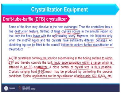
So, here I am having some more points about this. Some of the fines may dissolve in the heat exchanger and thus the crystallizer has a fine destruction feature because of the fine crystals.
