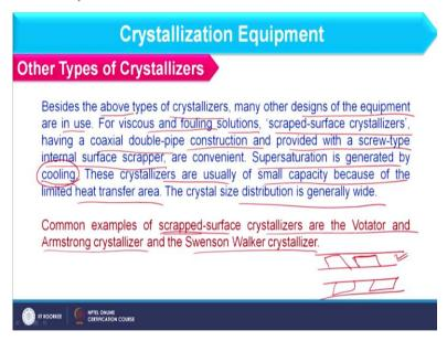
And we have some other type of crystallizer as besides the above type of crystallizer many other designs of the equipment are in use for viscous and fouling solution, scraped surface crystallizers are used which is having coaxial double pipe construction and provided with the screw type internal surface scrap. So, usually it is basically double pipe (()) (20:09) and at this outer surface of inner pipe we have this type of blade.
