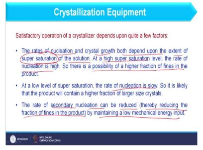
So, as far as satisfactory operation of crystallizer is concerned there are different factors on which it depends and these factors are the rate of nucleation and crystal growth both depend upon the extent of super saturation of the solution. So, how much super saturation is there the crystal formation depends on that. At a high super saturation level the rate of nucleation is high.
