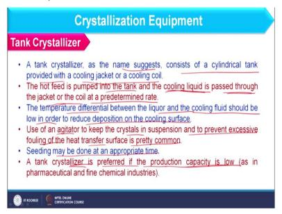
So, as far as this tank crystallizer is concerned as the name suggests it consists the cylindrical tank provided with the cooling jacket or cooling coil. So, usually it is a simple tank where either we can provide jacket or the cooling coil inside this. So, in this way it is called a tank crystallizer. So, the hot feed is pumped into the tank and cooling liquid is passed through the jacket or the coil at a predetermined rate.
