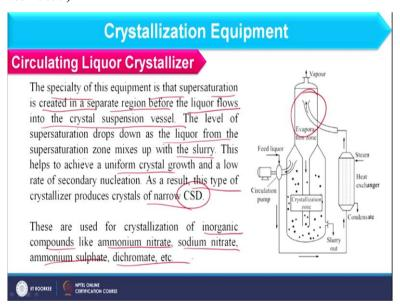
So, in this case the specialty of this equipment is that super saturation is created in a separate region before the liquor flows into the crystal suspension vessel. So, you can see here we can have the super saturation condition the level of super saturation drops down as the liquor from the super saturation zone mixes up with the slurry. So, this helps to achieve a uniform crystal growth and a low rate of secondary nucleation.
