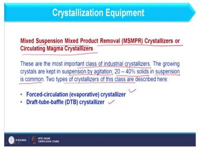
And let us see the equipment which are used in industry for crystallization. So, here initially I am considering mixed suspension, mixed product removal crystallizer for circulating magma crystallizer. So, these are most important class of industrial crystallizer. The growing crystal are kept in suspension with agitation and 20% to 40% solids in the suspension is common. So, in this category we usually have two types of crystallizer.
