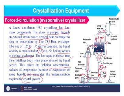
So, first of all I am focusing on forced circulation evaporative crystallizer. And as the name says it is forced circulation means it is using a pump to inlet the feed. So, feed is basically entering from here and it is mixed with the liquor which is exiting the crystallizer and both will enter into the heat exchanger. Here, temperature of the feed is increased, but not evaporation here only the sensible heat transfer occurs.
