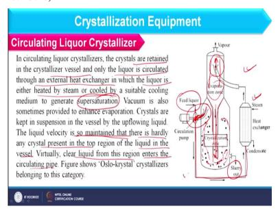
The schematic is shown over here. So, if you see here I am having the feed which is mixed with the liquor which is coming out from the crystallizer that is the mother liquor and it is mixed over here and then it is entering into the heat exchanger. So, superheated solution is entering into the vapour zone of this crystallizer and here evaporation takes place. So, in this case once evaporation happens because of the vacuum in the system the crystals and liquid is moving down.
