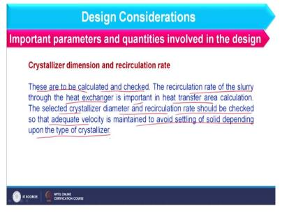
So, as far as crystallizer dimension is concerned it is basically the shell diameter and the height of the crystallizer. Height of the crystallizer means height of the shell of the crystallizer along with the tapered section because bottom section of crystallizer is usually tapered that also you have observed when we were discussing the working of crystallizer. So,
