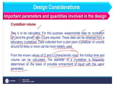
And further we have very important parameter that how to decide the crystallizer volume. So, as far as calculation of crystallizer volume is concerned we need the experimental data. Experimental data for what? Experimental data for nucleation and the crystal growth rate. So, nucleation that is B 0 and crystal growth rate that is basically G. So, in this way depending upon the solution we can find these data experimentally.
