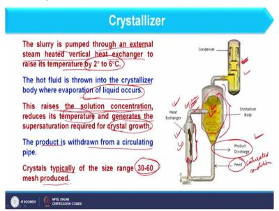
So, let us start with the working of crystallizer. So, as far as crystallizer is concerned it looks like this. So here we have some basic unit which are involved in crystallizer such as heat exchanger and here we have the condenser to condense the vapour and so it generates vacuum in the system. So, as far as working of crystallizer is concerned whatever solution is there that solution we consider as a feed and this is basically saturated condition.
