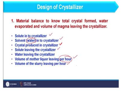
So, let us focus on design of crystallizer. So, as far as design of crystallizer are concerned we first consider on material balance and why material balance is required to know how much crystals are formed, how much water is evaporated and how much volume of magma as well as mother liquor which are leaving the crystallizer. So, let us see the steps involved in this. First of all, we should include the solute in the crystallizer that how much solute is entering into the crystallizer.
