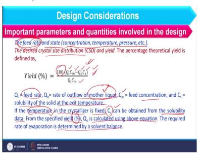
So, these are some important factors about design consideration now we will consider a few important parameters and quantity which should be involved in design of crystallizer. So, first is the feed rate and state means concentration temperature and pressure. So, that is very important parameter and secondly desire crystal size distribution and yield what should be the crystal size because we do not have a particular size of the crystal we usually have the range.
