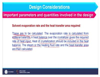
So, another parameter for design of crystallizer is the solvent evaporation rate and heat transfer area. So, solvent evaporation rate means it is occurring in the crystallizer and heat
