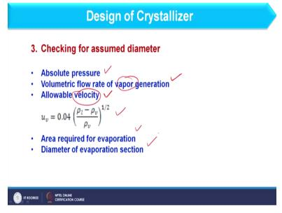
And to check that we will first consider the absolute pressure. What is this pressure? This pressure is corresponding to the pressure inside the crystallizer because usually the crystallizer is operated at vacuum pressure. Absolute pressure means atmospheric pressure minus the gauge pressure at which crystallizer is being operated. So, depending upon that we consider the absolute pressure.
