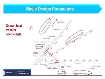
For that, we have this graph. In this graph, you see we have service fluid coefficient and process fluid coefficient. Now, what is service fluid, what is process fluid? Service fluid is basically that fluid which provides heat according to the requirement and process fluid is that fluid which temperature either increases or decreases as per the process requirement, fine. So, service fluid will be called when there will be the requirement from process fluid side.
