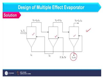
This is the flow sequence where feed is entering into second effect then to first effect and then to last effect. So, in this way final product exits from the last effect and that is L 3. So, usually XF and X 3 are known to you.
