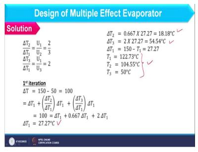
So, let us quickly cover the solution of this. We again have to find out temperature of each effect T 3 temperature is known to you. So, let us see the temperature of first and second effect considering equal heat transfer in each effect as we have discussed in previous example. So, I am not going into detail of that just see how the value can be obtained. So delta T 1 we can obtain as 27.27 degree Celsius delta 2 18.18 and delta 3 54.54. So T 1, T 2 and T 3 you can find accordingly as these.
