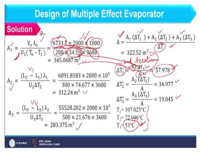
Here I am having area A 1 for first effect and that should be equal to V 0 lambda 0 that is basically the Q 1 divided by U 1 T 0 - T 1. So, you know all parameters V 0 should be given as kg per second when I am considering this balance. So, here it should be considered in seconds and lambda 0 is given as 2,000 and 1,000 because this is available in kilojoule and 200 is the U 1 value which is available in watt per meter square degree Celsius.
