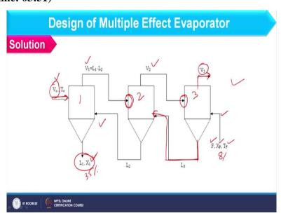
So, let us start the solution of this example here we are having the schematic where first, second and third effects are shown and feed enters into third effect because it is backward sequence with the flow rate F concentration XF and at temperature TF. So, when
