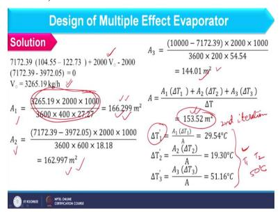
And so we can find out the steam flow rate that is 3265.19 considering the enthalpy balance of first effect and now we can find out area of each effect. So, area of first effect you can simply find out based on rate equation which comes out as 166.299 A 2 you can find out as 162.997 and so you can find out A 3 as 144.01 average area you can find as 153.52 from here you can see the deviation and so we require second iteration.
