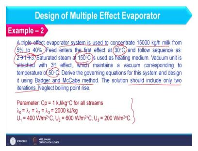
So, I am having second example also which I will cover quickly because here I am having different flow sequence. So, here again I have to design a triple effect evaporator system to concentrate 15,000 kg per hour of milk from 5% to 40% flow sequence is 213 that is basically the mixed. Feed enters at 30 degree Celsius, saturated steam is available at 150 and last effect temperature is 50.
