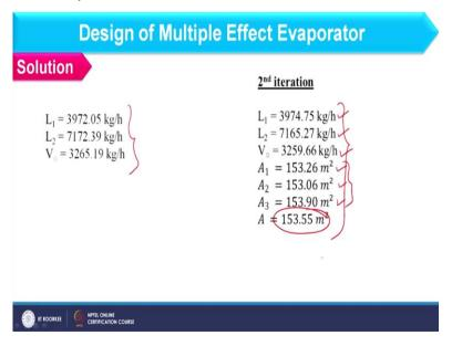
And so the result of second iteration you can compile as L 1 3974.75 L 2 7165.27 V 0 3259.66 A 1 that is area of first effect as 153.26 A 2 153.06 and A 3 153.9 and when you average it the average is pretty close to these value and that is 153.55, but still solution is not completed you have to iterate further. Till all six parameters of two consecutive iteration should be equal. So, in this way we can design triple effect evaporator system.
