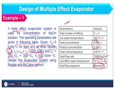
And in this example a triple effect evaporator system is used to concentrate sodium hydroxide solution, operating parameters are given in the table which is shown over here that we will discuss later on. In this case Cp of all feed as well as liquid streams are given as 3 kilojoule per kg degree Celsius. And latent heat of vapourization in each effect that is first, second and third effect along with the steam we are considering that as 2,000 kilojoule per kg.
