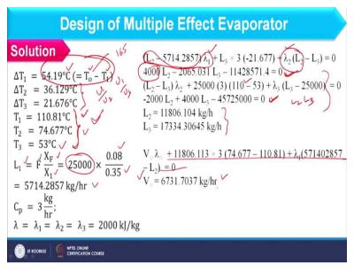
And so delta T 1 you can obtain as 54.19 degree Celsius and that should be equal to T 0 - T 1. Similarly delta T 2 and delta T 3 we can find out because I know delta T 1 and I know U ratios U 1 and U 2 or U 3 or U 1 / U 3. So, in this way I can find temperature of each effect. So, T 1 I can consider using this equation where T 0 is available at 165. So, considering this T 1 should come as 110.81 T 2.74.677 Celsius and T 3 will be 53.
