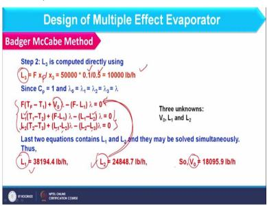
So, here we can make the component balance such as F XF should be equal to L 3 X 3 and feed and product concentration you know already. So you can find out L 3 value as 10,000 pound per hour. Now next you have to compute L 1 and L 2 because if you remember you have 6 parameters in which T 1 and T 2 you have already obtained. Now we have to compute L 1 and L 2.
