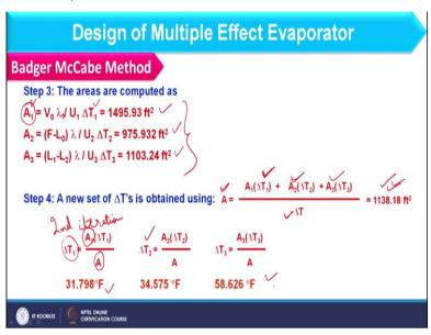
So, let us see the first effect rate equation so that should be equal to U 1 delta T 1 into A because now I am considering different area because area of each effect I have assumed as equal, but now we are considering different areas. So A 1 we can obtain as V 0 lambda 0 divided by U 1 delta T 1 so this value we can obtain like this. Similarly, I can obtain A 2 as well as A 3. So, area you can obtain like this.
