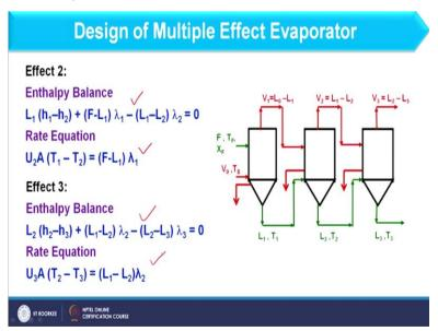
So, here we can have equation for second effect this is basically enthalpy balance of second effect and this is the rate equation. In the similar line, I can find equation for third effect also and we can have enthalpy balance like this and rate equation like this.
