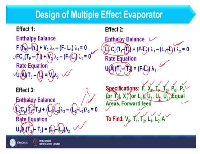
So, if I combinedly see equations of all effect we can observe that each effect is shown with two equation. We have total equation as 1, 2, 3, 4, 5 and 6 and here if you see we have further elaborated hF or h 1 what is the enthalpy of liquid that should be Cp of the liquid into temperature. So, considering that we have elaborated equation that is the enthalpy balance equation of all effects.
