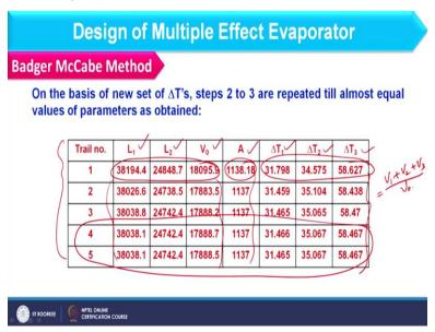
And results I have summarized as. If you see here I am having number of trials or the iterations and here I am having L 1 value, L 2 value V 0 A delta T 1, delta T 2 and delta T 3. So, if you see in first iteration I have observed values like this. This is the average area of first iterations and these values we already have seen in first iteration. So, if I change these temperatures the driving force you can further revise like this.
