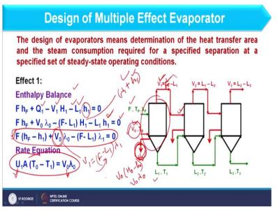
So, as far as triple effect evaporator is concerned this is the schematic where feed is entering into the first effect and concentrated liquor is entering from first to second effect and then to third effect and finally we have concentrated product from third effect. And similarly we can have the movement of vapour where steam is entering into the first effect and vapour generated in first effect is entering as a heating media in second effect.
