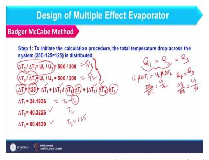
Now to find out unknown temperature we are taking another assumption that equal heat is transferred in each effect. So, if I consider Q 1 heat of first effect that should be equal to Q 2 and that should be equal to Q 3. If I am considering these two and elaborating it what we can observe U 1 A delta T 1 that should be equal to U 2 A delta T 2. So, here we are assuming that each effect area is same.
