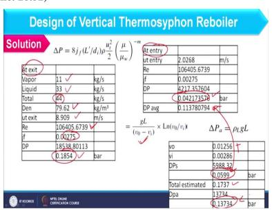
Now, let me calculate the pressure drop in tube side and that should be due to friction as well as static head. So, at exit condition of the tube we have this much vapour and 33 kg per second of liquid. So, total feed is 44. Density of the mixture comes as 79.62. This you can
