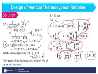
And next we have to find out the pressure drop due to static head and for that we have expression like this delta  $Ps = gl\ v\ 0 - v\ i$  into  $ln\ v\ 0\ / v\ i$  right. So, this  $v\ 0$  and  $v\ i$  are basically specific volumes and that will be nothing, but the reciprocal of density. So you can consider rho gl here, however, continuously phase is changed. So, we have consider specific volume instead of density.
