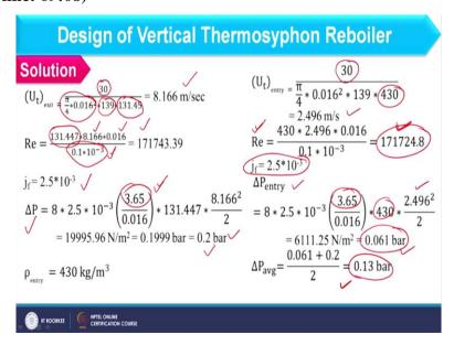
So, you see at exit condition total flow is 30 kg per second and here we have the mixture density because mixture is exiting the tube. Total flow area is basically 139 tubes into area of single tube. So, in this way we should find out velocity which comes as 8.166 meter per second. And if I know the velocity I can find out Reynolds number and here density of the mixture is considered and velocity is here and this is the tube ID.
