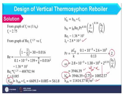
So, fs we will find out further as this expression in which we have to find out Reynolds number for the liquid and then fc we have already computed so we can find out fs value. So, Reynolds number for liquid we can find out considering 1 - x. So, you can see here because total feed is 5 in which 1 is vapour so 1/5 is the x value and total feed is given over here and we can find out Reynolds number like this which comes out as 1.38 into 10 is to the power 5.
