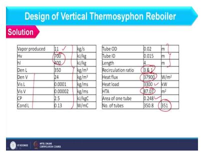
So, you see here I am having the values which are known to me that is 11 kg per second and this is basically the enthalpy of liquid and vapour and other properties and tube dimensions are given to us. Recirculation ratio is 3 is to 1, maximum reflux is 37,900 that we already have discussed that it is for vertical thermosyphon reboiler. So, accordingly we can find out heat duty depending upon vapour generation and latent heat of vapourization.
