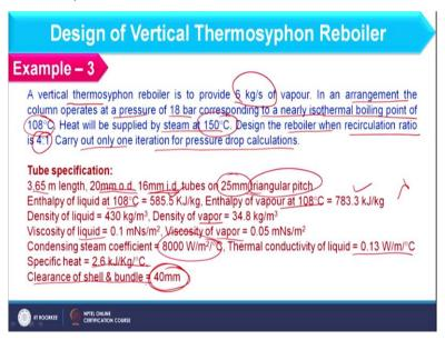
So, in this example a vertical thermosyphon is used where we have to generate 6 kg per second of vapour and if you recall the lecture of 6th week there we have discuss that in vertical thermosyphon reboiler boiling takes place only in tube side. So, that you have to keep in mind that in this problem also boiling is in tube side and the heating media is available in shell side.
