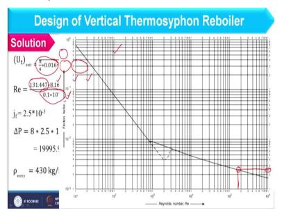
And we can find out jf factor from this graph where I have to locate 1.7 into 10 is to the power 5 so somewhere it will lie and this would be value of jf factor and you can see the value as 2.5 into 10 is to the power -3. So, once I am having all these value we can find out pressure drop due to friction at exit condition and in this case I am considering total tube length because whole length is available to provide frictional loss.
