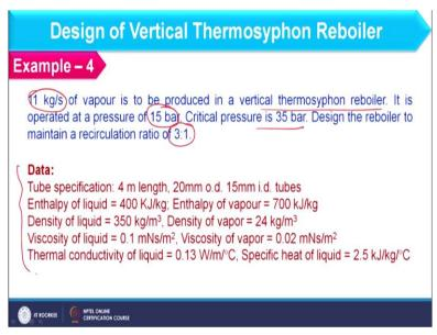
So, here you see we have 11 kg per second of vapour which is produced in vertical thermosyphon reboiler, operating pressure is 15 bar, critical pressure is 35 bar and here recirculation ratio of 3 is to 1 we have to maintain. Tube length and other properties are given I am not going into detail of these.
