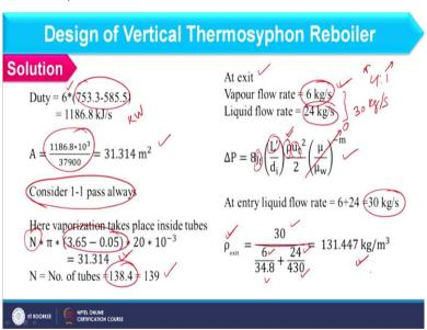
So, you see according to the problem we have 6 kg per second of vapour and this is basically the latent heat. So total 1,186.8 kilojoule per second or we can say kilowatt of heat duty is available. Now in vertical thermosyphon reboiler we have a different approach to find out area. Here we fix the maximum critical flux. Here we fix the maximum critical flux if you
