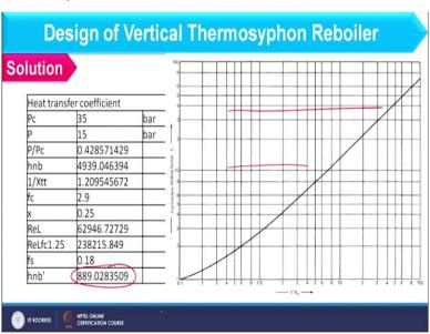
Now, heat transfer coefficient calculations are same as we have discussed in previous example so h nb dash you can find out as 889.03 watt per meter square degree Celsius. So, at exit point we have to find out pressure drop due to convective boiling.
