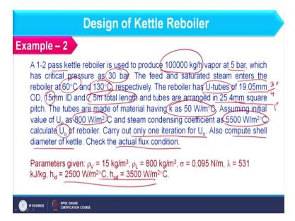
And here I am having second example which I will cover quickly. So, here you see 1-2 pass kettle reboiler is used to produce 1 lakh per hour of the vapour at 5 bar and critical pressure is 30 bar, feed and saturated steam enters the reboilers at 60 degree Celsius and 130 degree Celsius. So, in this case you see both are isothermal conditions. So, temperature difference should be difference of these two values.
