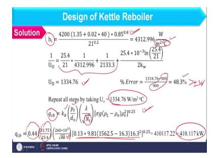
And so I can find out heat transfer coefficient in tube side considering this expression and so the value comes out as 4312.996 watt per meter square degree Celsius. So, as you have the value of h i as well as h 0 you can find out overall heat transfer coefficient calculation and in this problem dirt factors of two fluids are not given to us along with this thermal conductivity of tube material is also not known to me.
