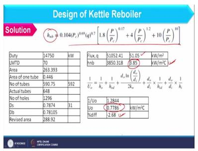
So, let us start the solution of this problem. Here, I have to find out heat duty that will be nothing but m lambda LMTD or we can say the mean temperature difference is 70 degree which is the difference of two temperatures only. Heat transfer area I can find out, area of one tube I can find out as we have discussed previously and number of tubes we can obtain as 592.
