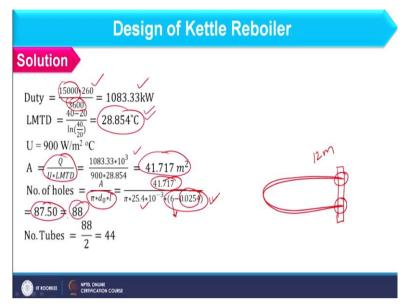
So, if you consider here heat duty is 1083.33 kilowatt where 15,000 kg per hour and that we have converted into seconds and 260 was the latent heat if you recall the example. Further, we have to find out log mean temperature difference because if you consider the temperature profile in chlorine side chlorine is entering at 10 degree Celsius and that is nothing, but the boiling point of the chlorine.
