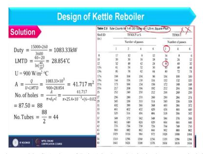
And further we have table C 5 where OD is 1 inch and 1.25 inch square pitch is given. So, as per the specification this table is suitable for me. So, let us see the actual tube count in this table. Here, I am having U tube and number of tubes we have obtained as 44 and passes are 2. So, if you see here I am having 44 tubes. So, in this case whatever number of tubes we have calculated the same number of tube is available in standard table.
