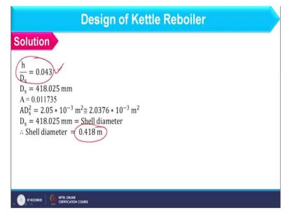
And we can obtain final diameter of shell as 0.418 and that is corresponding to h / D s value as 0.043. Now, if you recall the table 10 A where we have area sector factor. So, in that case only even values are available as far as h / D s is concerned so here we have to interpolate to find out the correct value for odd value of h / D s. So in that way you can design the kettle reboiler.
