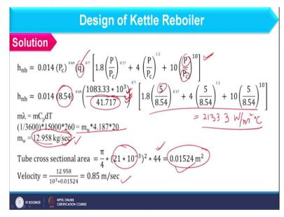
So, here we have the expression depending upon the critical pressure as well as the operating pressure along with the flux. So, what is this flux? This flux is nothing, but the heat duty divided by the heat transfer area. In this case whatever number of tubes you have obtained the same number of tube you can find in standard table C. However, if it will not happen then what you have to do?
