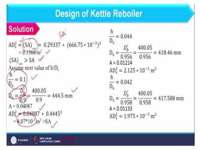
And further we can find out revised area as A into D s square. So, area we can obtain as 0.1304 that I am considering as SA calculated or you can simply consider that SA prime. So, in this case SA prime or SA calculated is very high in comparison to segment area. So, what we have to do further? We have to reduce the value of h? So, now we will consider slightly lesser ratio of h / D s.
