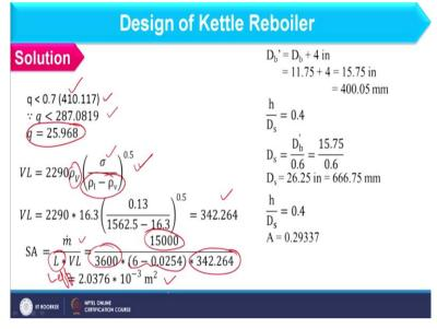
And what is the criteria for critical heat flux that the system heat flux should be less than 70% of critical heat flux. So, we should find out critical heat flux limit and that should be 0.7 into 410.117 so 287.0819 and system flux is this which is 25.968 kilowatt per meter square. So, you see the condition is satisfied here and next step is to find out the shell dia of kettle reboiler because here I am using special kind of shell.
