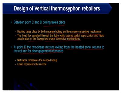
Further, if I consider the flow pattern between C and D here boiling will takes place. So, heating takes place by both nucleate boiling and two phase convective mechanism. Heat flux supplied through tube walls causes partial vaporization and rapid acceleration of the flowing two phase convective mechanism. So, as far as boiling is concerned we should consider nucleate boiling as well as convective boiling.
