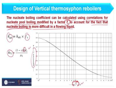
So, first of all we will focus on nucleate boiling coefficient. So that can be calculated considering the correlations for nucleate pool boiling which we have just seen in the last slide and that should be modified by a factor fs and this fs basically accounts for the fact that nucleate boiling is more difficult in flowing liquid because when we consider a nucleate boiling we understand that the fluid is at stagnant position, but here fluid is continuously moving.
