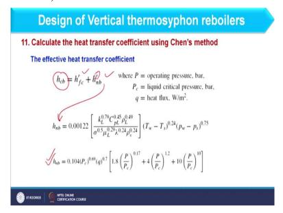
So, let us start the calculation of heat transfer coefficient using Chen's method. So, effective heat transfer coefficient should be what? Effective heat transfer coefficient at exit of the tube should be equal to h fc dash and h nb dash. So, h nb dash nucleate boiling coefficient you can find either by this equation or by this equation and here you see this is h nb we have to consider h nb prime.
