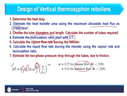
So, let us focus on the steps one by one. The first step is we have to define the heat duty or we have to compute the heat duty and how we can compute this because I already know that how much vapour I need to generate. So, that vapour flow rate into lambda will give me the heat duty and this is the simple calculation. So, once I am having the heat duty what we can consider next?
