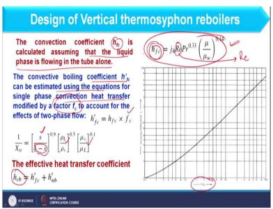
And further we have to consider convective coefficient because when liquid is available and vapour is available we have both mechanism of heat transfer convective heat transfer as well as nucleate boiling. So, convective coefficient that is h fc is calculated assuming that liquid phase is flowing in tube alone. So, here we have the correlation for convective heat transfer which we also consider in shell and tube heat exchanger.
