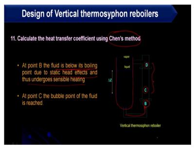
So, as far as heat transfer coefficient is concerned we find that through Chen's method. So, here I am having this vertical thermosyphon reboiler and I am having different points here like B, C and D. So, what will happen at point B? At point B fluid is below its boiling point due to static head effects and thus undergoes sensible heating. So, usually fluid enters to reboiler at boiling point, but because of some losses over here it may reach below boiling point.
