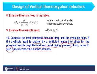
So, now we compare total estimated pressure drop and the available head. If available head is greater by a sufficient amount to allow for the pressure drop through the inlet and outlet piping we accept the design and proceed further if not we have to return to second step and increase the number of tubes. So, how I should increase the number of tube? In second step we have consider maximum heat flux.
