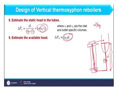
So, as far as static head is concerned we have the expression like rho g L, but here we are considering this differently because I am having different condition of feed at inlet as well as at exit condition. So, here we should consider specific volume instead of densities. So, you see here I am having specific volume at outlet and here I am having specific volume at inlet and this is nothing, but meter cube per kg.
