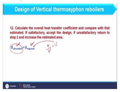
And shell side heat transfer coefficient you can find because steam will be available or if any other vapour will be available you can simply consider condensation process and find out heat transfer coefficient in that side. Once you have these two values, you can find out overall heat transfer coefficient and compare that with the estimated. So, you calculated you have already found from this thermosyphon reboiler calculation.
