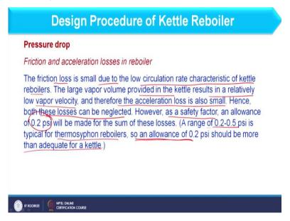
Now friction and acceleration losses in the reboiler: This we consider as the friction loss is small due to low circulation rate characteristics of kettle reboiler. The large vapour volume provided in kettle results in a relatively low vapour velocity and therefore the acceleration loss is also small. So, if we consider the friction and acceleration loss that is not significant. However, we consider that for safety purpose and we provide some losses to this section also.
