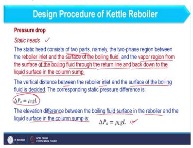
The static head consists of two parts such as reboiler inlet and surface of the boiling fluid. So, from the inner pipe to the liquid which; is available in the reboiler. So, from the inlet pipe to liquid which; is available in the reboiler because liquid will stay there. So, it will put some static head and further vapour region from the surface of boiling fluid through the return pipe and back down to the liquid surface in the column sump.
