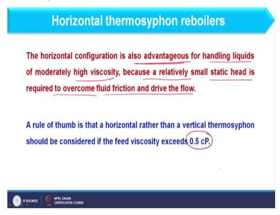
So, we have few more points about horizontal thermosyphon reboiler that horizontal configuration is also advantageous to handle liquid of moderately high viscosity because a relatively small static head is required to overcome fluid friction and drive the flow. When I consider horizontal thermosyphon reboiler it has less travelling distance by the fluid in comparison to vertical thermosyphon reboiler because vertical thermosyphon reboiler it has to travel the total length of the tube.
