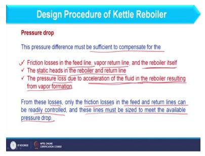
And further the pressure difference must be sufficient to compensate the followings. So, if you have the available pressure drop that pressure drop should be sufficient to consider the compensation corresponding to pressure drop in reservoir. So, the pressure drop we have obtained in column side that should be sufficiently high than the pressure drop, available in reboiler side.
