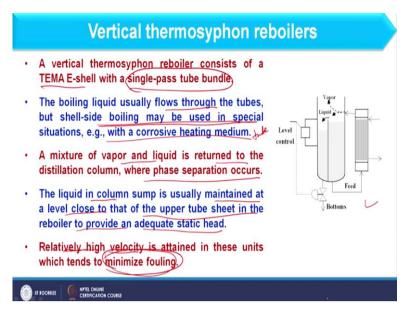
So, as far as vertical reboiler is concerned it consists of TEMA E-shell with single pass tube bundle. So, here you should keep in mind that passes in vertical thermosyphon reboilers are only one, one shell and one tube pass and that is quite obvious also because whatever vapour is generated it should move up, it should not move here and there in the exchanger and so the circulation cannot be maintained.
