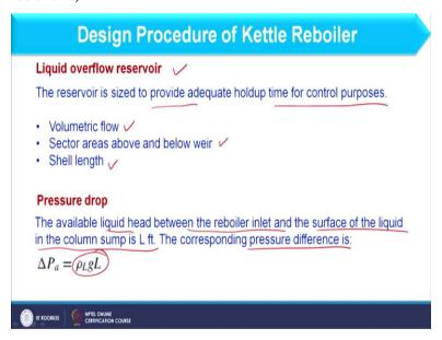
And now we will focus on the pressure drop part of the reboiler to ensure that liquid should come automatically from distillation column bottom to the reboiler. So, further design procedure of kettle reboiler says that we have to design liquid overflow reservoir. So, reservoir is sized to provide adequate holdup time for control purpose. And as far as liquid overflow reservoir is concerned we have to find out following parameters such as volumetric flow, sector area above and below weir.
