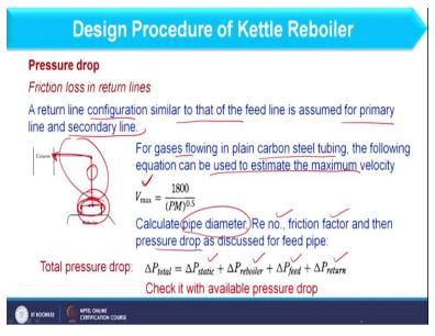
So, as far as return line is concerned again we have the nozzle from this vapour exits and it combinedly enters into the column so this is basically return line. So, the return line configurations similar to that of feed line consider primary as well as secondary line. So, this is basically secondary line and this is the primary line. In this case, we have gases not the liquid.
