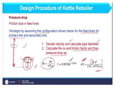
So, if you consider the feed line, feed line is basically this line because pressure drop which is available in this line that we already calculated and this we name as available head. Now, we have to find out friction loss in this. So, we begin by assuming the configuration shown here from the feed lines from primary line to secondary line. So, this is basically the primary line and these two are secondary line.
