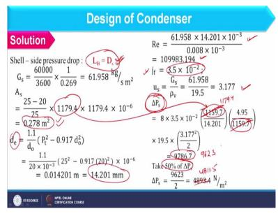
And now we will see the shell side pressure drop. So, to find out shell side pressure drop you have to fix the baffle spacing and that should be equal to shell diameter which is the specific change in construction of condenser and considering the vapour flow rate you can find out A s value because here you should consider Kern's method to find out pressure drop in shell dia.
