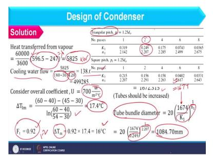
So, we are having 60,000 kg per hour of vapour and these are basically enthalpy of vapour as well as enthalpy of liquids. Difference of these two will give the lambda value and if you find it you can find 5825 kilowatt as the total heat duty of condenser. Once you have this heat duty you can find out flow rate of another fluid and that fluid is nothing, but the cooling water.
