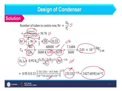
So, if you see the equation is given like this to us and here we have to find out gamma h this is not T h this is basically capital gamma h and further we have to find out N r dash. So, first of all let us calculate N r? So, N r will be what N r will be D b / P t dash. So, bundle diameter we have already obtained and that bundle dia will be divisible by P t dash and P t dash will be 0.87 into P t because I am considering triangular pitch.
