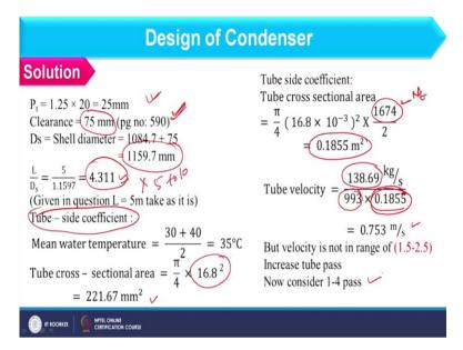
And after that we have to find out shell dia. So, to find out shell dia you should understand that clearance should be required and this clearance we can find out corresponding to bundle dia as well as the type of exchanger and that is the split ring. It is given already in the problem and that curve of clearance this you can find on page number 590 of Richardson Coulson volume 6 and it is from 4th edition of that book.
