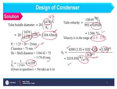
So, let us revise the bundle dia. Now, if I am having that bundle dia considering 1-4 pass you can find out K 1 and n 1 value according to triangular pitch and 1-4 pass you can have value as 0.175 like this as well as 2.285 like this. So, considering K 1 and n 1 value you can find out tube bundle diameter as this and further you have to see the clearance for spluttering exchanger and then you can find out shell diameter as 1179.43.
