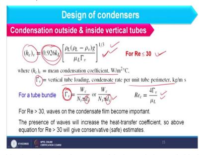
So, if you consider here I am having an empirical correlation and this is applicable for vertical tube rows. So, the expression is like 0.926 into different properties and here you see it is applicable for Reynolds number less than 30 where h c v is the mean condensate coefficient and gamma v is the vertical tube loading per unit periphery of the tube. For the tube bundle, we can consider gamma v which is equal to W c / N t pi d 0.
