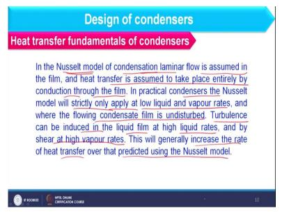
Further, if you see in the Nusselt model of condensation laminar flow is assumed in the film and heat transfer is assumed to take place entirely by the conduction through the film because we have the film and in this film we are not considering convection we consider that purely conduction will take place there. So, in practical condensers Nusselt model will strictly only apply at low liquid and vapour rates and where the flowing condensate film is undisturbed.
