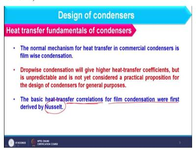
So, I hope all these fundamentals you know already and when we compare the film wise as well as drop wise condensation you should understand that heat transfer coefficient is more in drop wise condensation because of less resistance. However, the empirical correlations available for drop wise condensation is not as reliable as that is available for film wise condensation.
