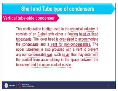
So, this configuration is often used in chemical industry. It consist of TEMA E-shell with either a floating head or fixed tubesheet. The lower head is oversized due to the accumulation of the condensate and vent for non condensable gases. So, if you see when I am considering vertical tube side condensation the condensate is collected from the bottom and at the same place we have to install vent nozzle.
