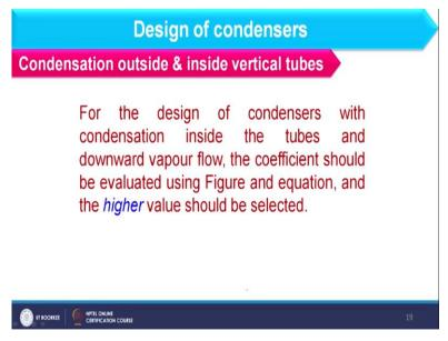
So, when I am considering inside vertical tube condensation you have to find out heat transfer coefficient using the graph as well as Boyko Kruzhilin correlation and consider the higher
