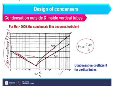
However, if I am considering Reynolds number in turbulent zone it means if Reynolds number is more than 2,000 we should consider this expression to find out heat transfer coefficient and here I am also having the Nusselt equation which is applicable below to Reynolds number 2,000 and after that it will depend on Prandtl number also. So, Prandtl number you can find out by this.
