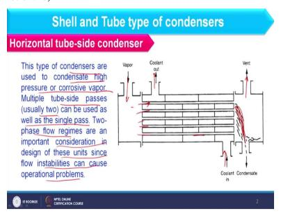
So, here you see I am having one schematic which you can understand as vapour is entering into tube side because here I am considering horizontal tube side condensation. So, vapour will enter in tubes and then from another side of the tube condensate exits. Now as far as
