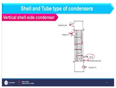
Now, if you see the schematic there you can understand it properly that vapour is usually enters from the top and it does not space to move upward because here we have end of the shell. So, vapour will move downward along with the condensate. Now in this case baffle cut is usual as we consider in normal shell and tube heat exchanger and as condensation process proceeds condensate moves downward.
