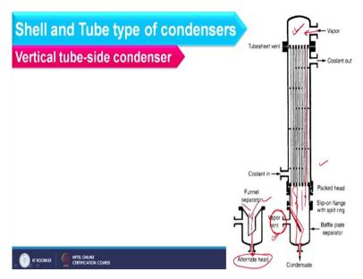
And now we will focus on the schematic. So, if you see the schematic of vertical tube side condenser vapour usually enters to tubes side from the top and moves downwards along with the condensate and if you see this section is oversized in comparison to this section where I am having condensate as well as the vent because vent is usually placed opposite to the side where vapour is entering.
