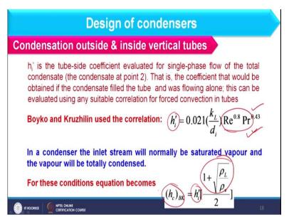
So for that case Boyko Kruzhilin consider the expression of usual heat transfer coefficient which you also have seen in sensible heat transfer and this is given by h i dash and this expression you can use which is the function of Reynolds number and Prandtl number and when I am considering that saturated vapour is entering and complete condensation is occurring at the end of the exchanger.
