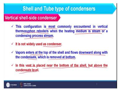
Now we will discuss vertical shell side condenser. So, you see this configuration is most commonly encountered in vertical thermosyphon reboilers. So instead of condenser, we consider vertical shell side condensation in thermosyphon reboiler. So, in that case boiling will occur in tube side. So, this point we will further elaborate when we will focus on the topic reboilers.
