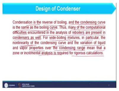
Now, let us further discuss few facts about condenser. So you see condensation is a reverse of boiling, boiling we generate vapour and in condenser we generate liquid and the condensing curve is the same as the boiling curve. Thus, many of the computational difficulties encountered in the analysis of reboilers are present in condenser as well because both activity are just opposite to each other if I consider reboiler and if I consider condenser.
