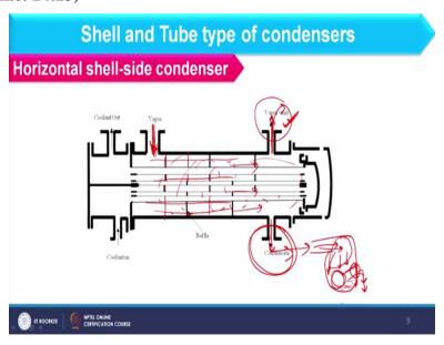
So, here we have the condenser and here vapour is entering into the shell side and if you see in this case baffle should be like this because we have vertical cut in baffles. So, vapour is entering into the shell side and from here at the bottom we have condensate removal continuously. Now, what we have discussed previously that it has one extra nozzle and that we can call as vent so that you can see here I am having a vent which is just at the end of the exchanger.
