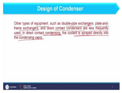
And apart from that other type of exchangers are also used, but it is used as a condenser is not significant. However, other type of equipment such as double pipe heat exchanger, plate and frame exchanger and direct contact condensers are less frequently used. However, it is used, but use is not extensive. In direct contact condensing coolant is sprayed directly into the condensing vapour.
