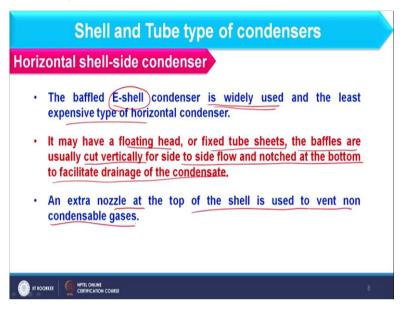
So, now discuss few more points about horizontal shell side condenser and here we usually consider E- shell so TEMA E-shell is considered over here and it is widely used in a condenser and the least expensive type of horizontal condenser so that you can understand because TEMA E is the simplest type of shell so that becomes inexpensive also in comparison to others and therefore it is widely used in condenser.
