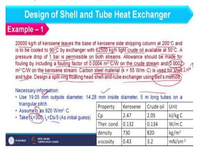
So, let us start this. So, here I am having example 1 and in this example we have 20,000 kg per hour of kerosene which exits the base of kerosene side stripping column at 200 degree Celsius and to be cooled to 90 degree by exchanging heat with 62,500 kg per hour of light crude oil which is available at 50 degree Celsius. A pressure drop of one bar is permissible on both streams.
