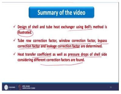
So, in this video design of shell and tube heat exchanging using Bell's method is illustrated with the help of one example where tube row correction factor, window correction factor, bypass correction factor and leakage correction factors are determined and finally heat transfer coefficient as well as pressure drop in shell drop considering different correction factors are found.
