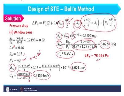
Now we have to find out pressure drop in window zone. So, this is the expression for pressure drop in window zone. Here I have to find out N wv and U z and U z is basically the
