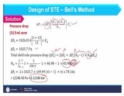
And further we have to find out pressure drop in end zone and the expression for that is given over here where N wv is 5 and N cv is 13 delta P i we have already calculated previously. So considering all these values, you can find out delta P e as 1025.7 pascal. So, total shell side pressure drop that is delta P s should be equal to 2 into delta P e because we are having two end zone.
