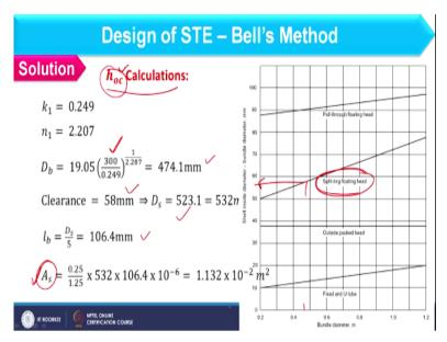
So, the first step is to find out hoc. So we have to consider calculations for hoc and this hoc will depend on us and gs value which is as per Kern's method. So, first of all we should find out As value and for that we should calculate baffle spacing and shell dia. So, to find out shell dia we should first find out the bundle dia depending upon the arrangement and the passes. So here I am having 1-2 pass and arrangement is triangular.
