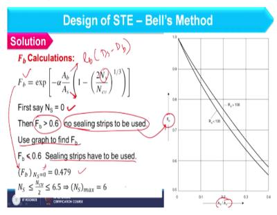
So as far as bypass correction factor is concerned here we have the expression for F b where number of sealing strips are given as N s. So, first of all we should find out whether sealing strips are required or not and to calculate that we should consider N s = 0 in this expression and to find F b value. So, considering N s = 0 we can find out F b based on A b and A s value. A b is basically the baffle spacing into D s - D b.
