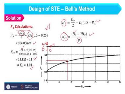
Now once you have h oc value we should find out other correction factors and let us see how to find out F n F w F b and F L. So let us start with F n value. So here I am having F n calculation and you have already seen that fluid is falling in turbulent flow. So we have to use the graph of F n for which N cv should be known to me. So to find out N cv we should consider H b. So first of all I will find out H b using this expression.
