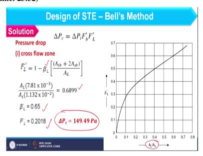
Now we should quickly cover pressure drop in shell side. Now as you know that pressure drop we should consider in cross flow zone, window zone and end zone separately. So let us
