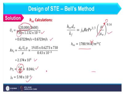
So, velocity of shell side you can find considering kerosene flow rate because that is allocated to shell side only its density as well as A s value considering all these you can find velocity in shell side at bundle equator as 0.6723. Now, if you see this problem here we are already given the properties because the collection of property we have already discussed in Kern's method in detail and in the similar line you can find the properties of the fluid.
