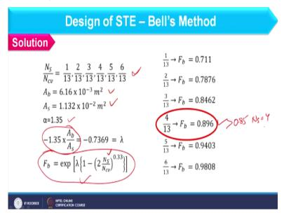
So, let us see the calculations if I am having N s and N cv like 1 / 13, 2 / 13 in this way. So further we can obtain A b and A s which we have already used in F b calculation in the last equation and here alpha value should be used as 1.35 depending upon the flow. So in this case we can consider this term in the expression as lambda and we can further reduce the F b expression like this where it is the function of N s and N cv.
