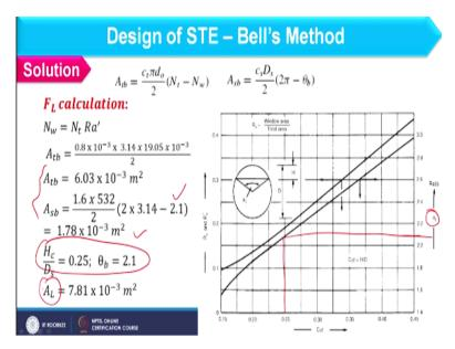
So as far as leakage correction factor is concerned we should calculate A tb and A sb so A tb and A sb expressions are given over here and here we require N w so N w should be N t into R a dash R a dash we have already calculated and A tb you can find out using this expression where c t is basically clearance between hole in baffle and tube OD. So this c t is always equal to 0.8 mm so in this way you can find out A tb value.
