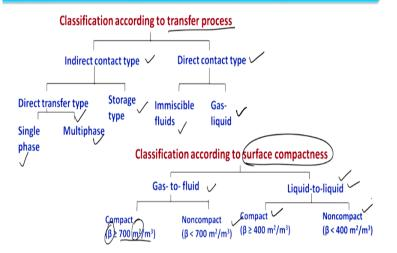
Now, we will focus on classification of heat exchangers and these classification depends on different factors. So, the first factor is we are going to classify the heat exchanger based on transfer process, how heat is transferring from one fluid to another fluid based on that we are going to classify. So, if you focus on this when I am considering transfer processes based on that, we have indirect contact type and we have direct contact type.
