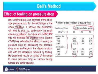
So Bell's method gives an estimate of shell side pressure drop for the exchanger in clean condition. In service the clearance is tend to plug up particularly in small clearance between tubes and baffle and this will increase the pressure drop and therefore we can have one table where ratio of foul to clean pressure drops are shown depending upon the baffle spacing and the regions.
