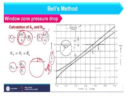
So here we should consider the calculations of A w and N wv. So as far as A w is concerned that is basically what is A w? A w is basically free area which is available for fluid to move in window zone. So how I can consider that? If you see the expressions goes as pi D s square / 4 so that is nothing, but the cross sectional area of shell and what is R a? R a we have already discussed in lecture 2 and lecture 3 of this week.
