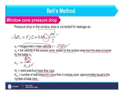
So, when we focus on pressure drop in window area or window zone this is the expression delta P w is equal to F L dash 2 + 0.6 N wv rho u z square / 2. So here as far as u z is concerned this is the geometric mean velocity of which velocities? The velocity which is occurring in cross flow zone and velocity which is occurring in window zone. So, that should be the geometric mean of u w as well as u s that is for cross flow zone that you have already seen in Kern's method.
