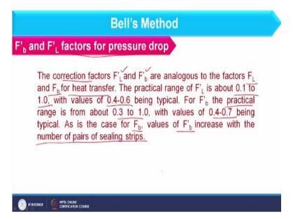
Now here we have F b dash and F L dash factors for pressure drop and here we are going to understand the range of these factors. So, the correction factors that is F L dash and F b dash are analogous to factors F L and F b for heat transfer that we have already discussed. Now the practical range of F L range is about 0.1 to 0.1 with values 0.4 to 0.6 being typical. So, it will be better if value will lie between 0.4 to 0.6.
