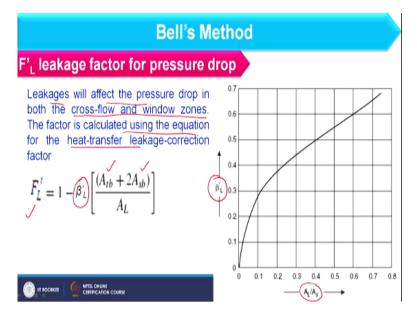
So, further we should understand F L dash that is leakage correction factor for pressure drop. So leakages will affect the pressure drop in both the cross flow as well as window zone because in cross flow zone again we have the leakages between baffle hole and tube OD and in window zone we have leakage between shell dia and baffle dia. So, between that space we can find leakages.
