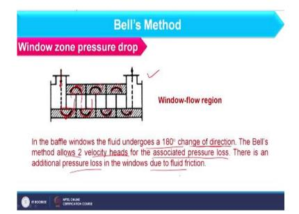
So, first see what is window zone? If you consider this schematic here fluid is entering and we have already considered the section which are falling between baffle tips that we consider as cross flow zone. However, we can consider the zone which is available between baffle tip and shell diameter so that zone basically we can call as window zone as showing in this schematic through shading.
