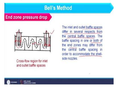
And now we will focus on end zone pressure drop. So, as you can see here we have end zone where fluid is entering and from where fluid is exiting these zones we are considering as end zones. So the inlet and outlet baffle spaces differ in several respects from central baffle spaces like whatever spacing are there in between here spacing will be slightly different as you can observe from this image also.
