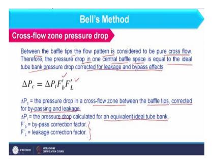
So, let us see the cross flow zone pressure drop how we should obtain that. So, what should be the pattern in cross flow zone pressure drop? We can understand that between the baffle tips the flow pattern is considered to be pure cross flow. Why it is cross flow because in tubes fluid is moving horizontally and when shell side fluid will come between two baffle tip it basically moves perpendicular to the tubes and therefore it is called as cross flow.
