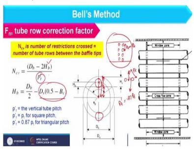
So first of all we have to find how to compute N cv and so we can calculate F n that is tube row correction factor. To understand that, we consider this schematic where number of tube rows are basically these so that is available between two baffle tip one tip is this, one tip is this and here we have this window zone and in between baffle tip we consider cross flow zone.
