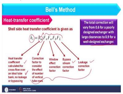
Here in this expression you can see here I am having shell side heat transfer coefficient, here I am having h oc and then we consider different factors. So, let us see what these are? H oc is basically heat transfer coefficient calculated for cross flow over an ideal tube bank where no leakage and bypassing are there. So, once I am calculating h oc after that we will consider different factors such as F n.
