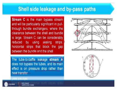
So, if you see when I am considering stream C this is only the bypass stream which is available in shell side and that stream is more significant when I am considering pull through bundle exchanger or internal floating head as we have discussed in lecture which is on classification of heat exchangers there we have discussed that main limitation of internal floating head heat exchanger it is having more shell diameter it means it has more clearance.
