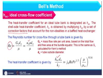
So, the heat transfer coefficient of an ideal tube bank is designed as h oc. The shell side heat transfer coefficient h s is obtained by multiplying h oc by different correction factors to consider non idealities in baffled heat exchanger or the shell side of heat exchanger. For that we have to calculate Reynolds number for cross flow through a tube bank and Reynolds number is basically the function of shell side velocity density d o and mu.
