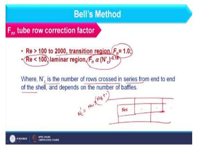
So in that way we can find out the N cv and so in that way we can find N cv value and you can refer the previous gap to find out F n value, but that will be applicable when Reynolds number is more than 2,000. Now what will happen when Reynolds number is 100 to 2,000 that we consider as transition region in shell side in that case F n should be taken as 1 you do not have to do anything.
