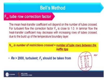
So, first of all I am considering tube row correction factor and that I am representing as F n and in the book same nomenclature is used. So the main heat transfer coefficient will depend on number of tubes crossed means what when the flow is occurring in tube side shell side flow should be perpendicular to that. So, whatever number of tubes are available fluid should pass that tubes and that tube we consider as tube row.
