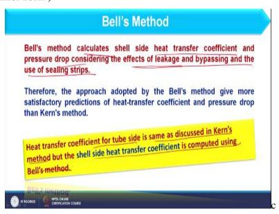
So, let us start the Bell's method. So Bell's method calculates shell side heat transfer coefficient and pressure drop considering effects of leakage and bypassing and the use of sealing strips. So we will discuss all these factor in Bell's method how it will be applicable. So, if I am comparing this method with the Kern's method obviously Bell's method gives more satisfactory result in comparison to Kern's method.
