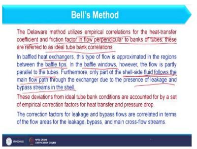
So as far as Bell's method is concerned this method utilizes empirical correlations for heat transfer coefficient and friction factor in flow perpendicular to banks of tubes. These are referred to as ideal tube bank correlation. So, the Bell's method first consider ideal tube bank.
