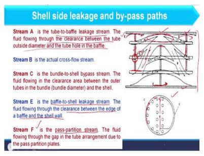
So, here we will discuss shell side leakage and bypass paths. So what are the different streams which are related to shell side that we are going to discuss now. Now, if you see this is the schematic where this is shell and these sections are basically baffles and we have different streams like E, A, B like that and other streams also which are not showing over here that I will discuss.
