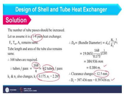
For 1-4 pass what change I have to do? So 1-4 pass what changes we have to carry out? First change is when I am considering the bundle dia because for 1-4 pass k 1 and n 1 value will change and once I am having this we should also find out the correct tube numbers. Though, I have already find out as 166 in 1-2 pass now for 1-4 pass if you divide 166 / 4 the value will come in decimal so that is not acceptable for tube.
