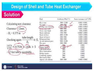
So in this table we can consider organic liquid and benzene will fall in this category. So we have coefficient as 5,000 for benzene cooling tower water the range is given as 3,000 to 6,000 so we have to take the average length so here we can have the value 4,500 and 5,000 for benzene. So, if you see heat transfer coefficient is less for water it means dirt factor is more for water. So, water should be allocated to tube side and benzene is allocated to shell side.
