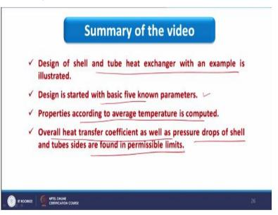
And now I am having the summary of this video and here design of shell and tube heat exchanger is illustrated with the help of one example. Design we have started with basic five known parameters that I have already discussed. Properties according to average temperature is computed and I have already explained how you can obtain these properties and finally overall heat transfer coefficient as well as pressure drop of shell and tube side are found in permissible limit.
