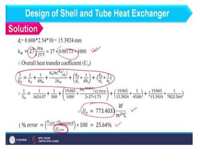
So I can calculate overall heat transfer coefficient because you know dirt factor of both fluids and you also know the thermal conductivity of the material. So that thermal conductivity you can assume as 27 and when I convert it I can find the thermal conductivity like this and you put all the values in this expression and overall heat transfer coefficient you can find as 773.4. I should compare that with assumed value should come.
