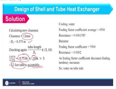
Considering clearance from the same manner as we have discussed in the last iteration. Diameter of shell is equal to 0.375 and L/D ratio will come as 9.7536 so that should be less than 10 so we can consider that 12 feet tube length is acceptable. So, in this way you have
