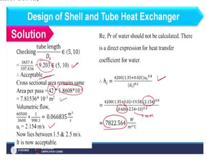
So, once I am having this shell dia we can again check L / D ratio every time we have to do this because we should also ensure that optimum ratio should be obtained. So if I am doing so I am finding L / D ratio as 9.203 which is in the range and so the length and diameter is acceptable. So, next is we have to find out the right velocity and for that we have to calculate area per pass.
