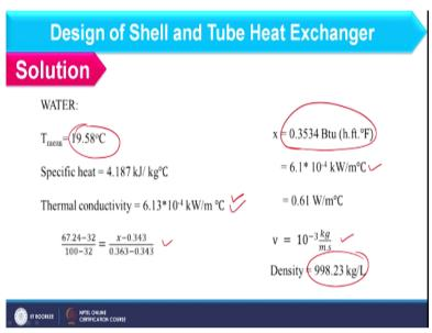
In the similar line, I can find out the thermal conductivity of water. So, you can see average temperature is 19.58 which can be converted into Fahrenheit and thermal conductivity we can obtain by this and thermal conductivity of the water we can find as 6.13 into 10 to the power –4. Now how I will obtain that? Let us see the thermal conductivity table. So, this is the table where for water I am having complete range of temperatures and accordingly thermal conductivity is given.
