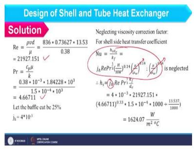
So, considering all these value we will find out the Reynolds number and then the Prandtl number and then we will consider the heat transfer coefficient expression and which is basically this for shell side. So, here I am neglecting this term that is the viscosity correction factor so this I should not consider and here we have to find out j h value.
