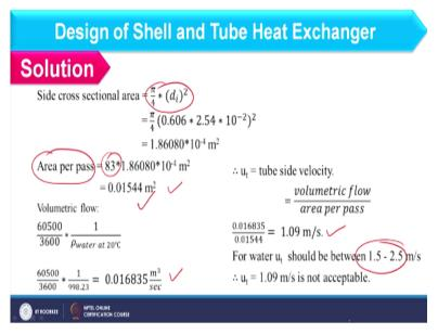
Now, if you have allocated the fluid to shell side and tube side you have to find out heat transfer coefficient of tube side as well as shell side. So, first of all we will calculate that for tube side and to carry out that we have to find out the velocity and for velocity I have to choose cross-sectional area of single pass. So for that we can consider cross sectional area of a single tube.
