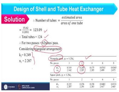
Now once I am having the area of one tube I can simply calculate number of tubes because I already know the heat transfer area. So, the calculation gives 123.09. As I am having 1-2 pass the tube number should be even. So I am considering 124 as total number of tubes, two passes I am considering so 62 tubes will be available in one pass. So considering the two pass and assuming triangular arrangement.
