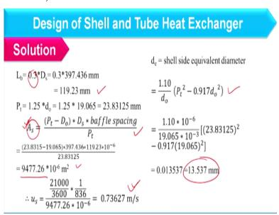
Now, next step is what? Next step is to find out heat transfer coefficient in shell side and to carry out this we have to specify baffle spacing. So, the baffle spacing if you remember the optimum range varies from 0.3 to 0.5 into shell dia. So, here I am considering 0.3 into shell dia. So, baffle spacing comes as 119.23 and here I am considering Kern's method for heat transfer coefficient calculation in shell side as well as pressure drop in shell side.
