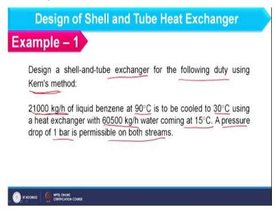
So, let us start the design of shell and tube heat exchanger using Kern's method with the following example. So, here I am having example 1 in which design a shell and tube heat exchanger should be carried out for following duty and that design I have to do using Kern's method. 21,000 kg per hour of liquid benzene which is available at 90 degree Celsius is to be cooled to 30 degree Celsius.
