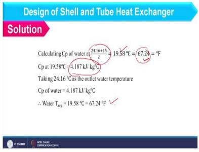
And then we carry out the averaging of the water which is coming as 19.58 degree Celsius and that should be 67.24 degree Fahrenheit. Now at this average temperature, we again have to see the C p value from the graph which will come out as 4.187 so in the case of water the assumption will be equal. However, that will be completely iterative approach when you are considering the other fluids than the water and there is no guideline to assume initial C p value that randomly you have to assume.
