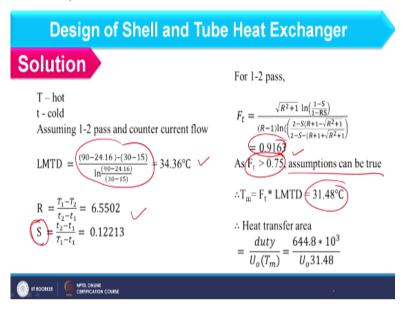
So, simple LMTD expression you know so that we will apply over here and 34.36 degree Celsius we have obtained. So, as it is the LMTD for counter current flow we have to carry out shell and tube heat exchanger design where at least one, two pass I should consider. So in that case F t correction factor should also be included. So, for that purpose we have to find out R and P value.
