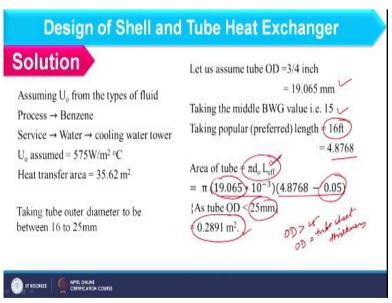
So, the value of overall heat transfer coefficient you can obtain 575 as initial guess so heat transfer area you can calculate as 35.62 meter square. Now we have to decide the tube
