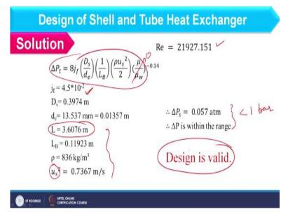
Next, we will consider the pressure drop in shell side for that you have to use this expression considering neglecting viscosity correction factor and for this Reynolds number which we have already calculated to 2.2 somewhere here and this is 25 baffle cut. So, you can find out the value of j f at this point which will be around 0.5 into 10 to the power -2 which will be around 4.5 10 to the power -2.
