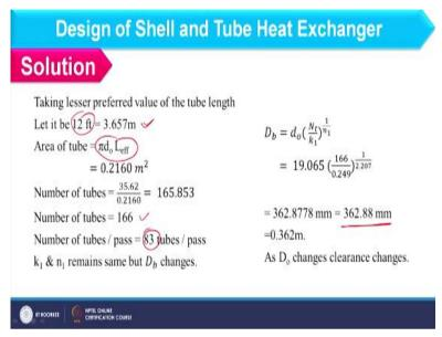
So, here I am considering L effective based on 12 feet meter length which will be equal to 3.657 meter. In this case number of tubes will be 166 because I have to consider even number so 83 tubes will fall in each pass. So, accordingly I can calculate bundle dia.
