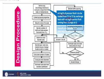
So, let us start with the first step that is define the duty. Now to define this duty we should understand that what are the known parameters to me. So, the problem of shell and tube heat exchanger design goes as m 1 kg per hour of the process fluid is to be cooled from T 1 to T 2.
