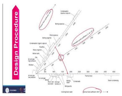
Now how I have to assume this that you can do through this graph which I have already discussed in basic design parameters. So here I am having the process fluids and here I am having the service fluids depending upon the process fluid and service fluid you can consider the center of these ranges whatever fluids you are considering and just draw a line between the two.
