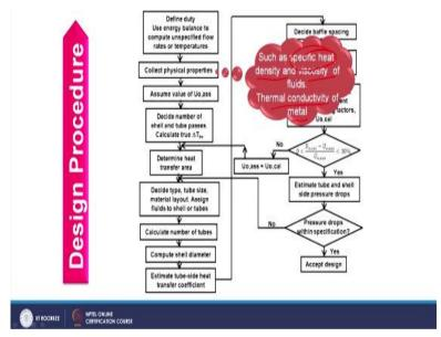
And physical properties such as density, viscosity of the fluid, thermal conductivity of the metal and for the fluid because specific heat you have already calculated and how you have to calculate this and how you have to collect the physical properties which we have already discussed in double pipe heat exchanger design just I am giving an overview.
