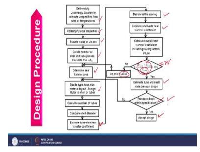
Let us see the procedure for design of shell and tube heat exchanger and what are the steps involved this one by one. So, the very first step is to define heat duty of the exchanger and use energy balance to compute unspecified flow rates or temperature. So, if you see here we have unspecified flow rates and temperature, what is the unknown parameter and what are the known parameter that we will discuss in details of this design.
