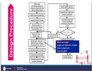
And once you have this overall heat transfer coefficient which is obviously the assumed value heat duty and true LMTD you can simply calculate heat transfer area. So, that is basically the total heat transfer area of the exchanger and after that you need to decide the following parameters such as decide type, tube size, material layout, assign fluid to shell side or tube side. So which exchanger you have to choose how you can decide that?
