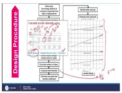
And after that you have to find out shell diameter and to calculate the shell diameter you first need to calculate the bundle diameter which you can calculate from this expression where d 0 is the outer diameter of tube N t is total number. So it will not depend on the passes whatever number of tubes you have obtained just check that it should be even number so that N t you can consider over K 1 and N 1 will depend on the passes as well as the pitch.
