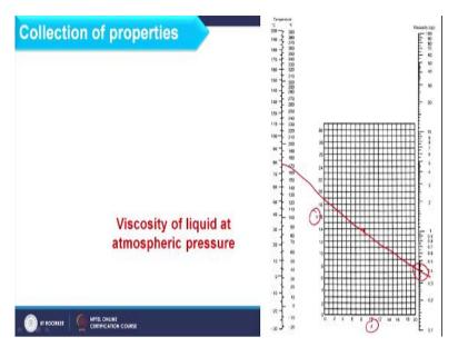
Here you can see the viscosity data and X and Y are given to you. So these X and Y you can find from these tables we have discussed all these in detail in double pipe heat exchanger. So, according to the X and Y value you can place a mark in this and depending upon the average temperature whatever it is you can simply make a line crossing that point and wherever it is cutting the right axis that value you can note as the viscosity of the fluid.
