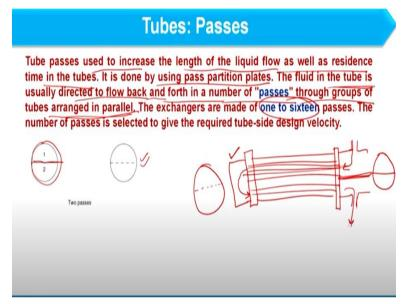
So if this is the complete cross section of the shell, and this we have divided into part and if I see the dotted line, dotted line shows that on another side of heat exchanger, we have the pass. To give an example if this is the fixed tube sheet, okay. This is the heat exchanger. And let us say here I am having the cover, right. And here I am having the tubes, okay. And pass partition plate is available here.
