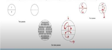
And now we will focus on the passes, okay. If I consider tube pass, what is the meaning of this? Basically I am dividing the fluid okay which is entering in the tubes and let us say if I am having 100 tubes, the complete mass flow rate of fluid which is allocated to tube side will be entered to 100 tubes in single time, okay. Now if I consider tube pass and if I consider one tube pass, what is the meaning of that?
