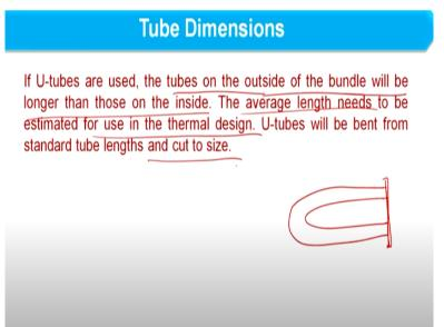
If I am having tube sheet like this, okay. Here I am having inner tube and if I am considering outer tube, it means outer tube dimension or size is very large in comparison to inner pipe, right. So the average length needs to be estimated for the use in thermal design, okay. So U-tube will be bent from the standard tube length and cut to the size. So in this way we usually consider the U-tube.
