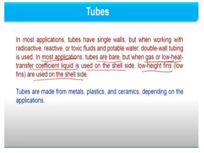
In most applications, in most of the application, we usually consider tubes with single wall, but for special consideration where I am dealing with radioactive material, I am dealing with where I am dealing with radioactive material, I am dealing with toxic fluids, we should we can use double walled tubes also, okay. So tubes are both single wall as well as double walled. And in most of the application tubes are bare.
