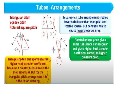
Now next we will discuss the tube arrangement, how tubes are arranged, okay. The first one is the triangular tube, the first one is the triangular pitch. So this is the schematic of triangular pitch. Now what is the pitch? Pitch is basically the distance between center to center line of two consecutive pipes, okay center to center lines of two consecutive pipes. So that is basically the pitch.
