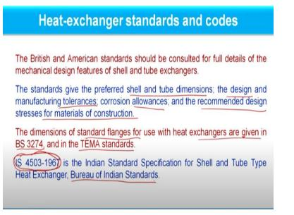
So British and American standards should be consulted for full details of mechanical design feature of shell and tube exchanger. So if you see all these codes, which are
