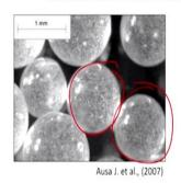
Expendable polystyrene is produced via suspension polymerization in the presence of the blowing agent (pentane).
