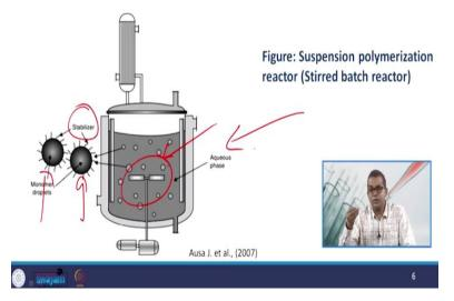
This is the aqueous phase and these are the monomer droplets and with the help of certain stabilizer and stirrer. So, this is the stereotype of a batch reactor and this type of approach is very common for the synthesis of polymeric beads. And these polymeric beads are usually the crosslink polystyrene beads. They are very good support for the catalytic or some they are used for the different type of supports for the ion exchangers.
