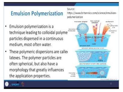
So, you can see that here we are introducing the monomer droplets. There are certain free radical initiators if you recall that to initiate the polymerization process, you will require certain type of induced material. In this case, the induced material is free radical initiator and sometimes, because we are using the water as the continuous dispersion media, you may require some surfactant to alter the surface energy of water.
