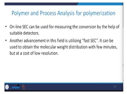
Now, sometimes the online size exclusion chromatography is very popular. And this can be used for the measuring of conversion by the help of suitable detectors. Now, it offers another advantage in the field that is utilising the fast size exclusion chromatography or SEC. Now, it can be used to obtain the molecular weight distribution within a few minutes, but at a cost of very low resolution.
