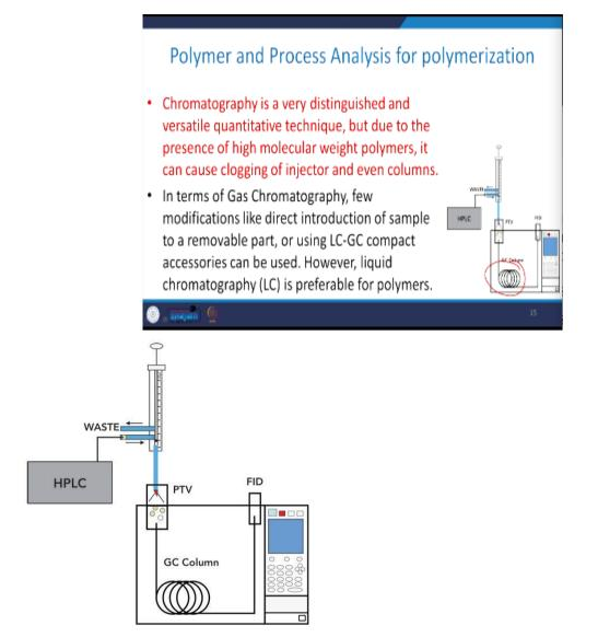
Now, when we talk about the chromatographic techniques, it is a very distinguished and versatile quantitative technique, but due to the presence of some high molecular weight polymer, it can also clog the injector or even columns. See, just I am giving you a brief about this particular chromatographic technique. As you see in this particular thing, there are very small openings or very small diameter columns.
