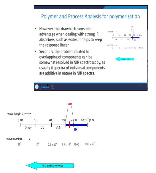
Usually, to keep the response in a linear range, as quite visible in this particular figure. Now, secondly, the problems related to overlapping of component, it can be some somewhere resolved in these types of infrared spectroscopy things. As these a spectra of individual component, they are sometimes additive in nature when we talk about the domain of near infrared. So, this is again a good aspect related to the NIR thing.
