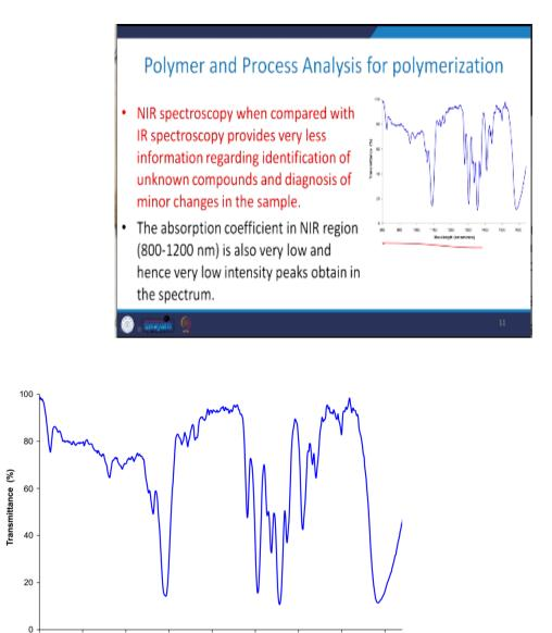
Now, the absorption coefficient in the range of NIR range of 800 to 1200 is very low. And there is the very low intensity peaks, you may obtain in that particular spectrum as it is visible in this particular plot. However, this drawback because, it is sometimes, people feel that this is a drawback. So, when we talk about this thing, then this drawback turns into advantage when you are dealing with strong infrared absorbers such as water.
