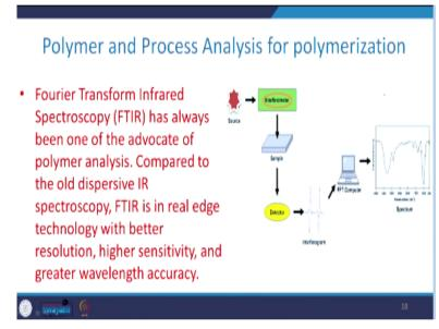
Here, a schematic diagram represents the basic concept of FTIR, you are having the interferometer. So, the source may be like this and then it passes through the sample that is infrared. And there is a detector who analyses and by this way, you may get the interferogram and which you can analysed with the help of computer to get this particular spectra.
