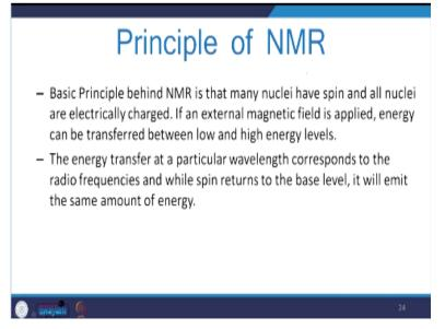
So, if you apply the external magnetic field, the energy can be transferred between low and high energy levels. So, these 2 levels are there. So, it can be transferred between these 2 energy
