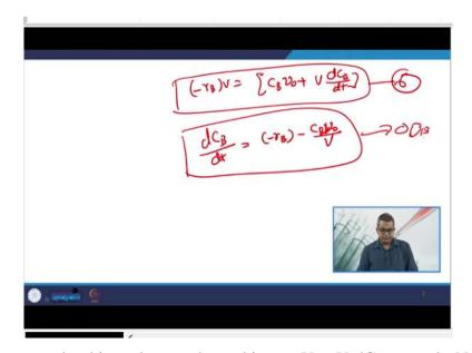
And if we rearrange the things then we have this -  $r_B V + V dC_B$  upon dt. Now, this is my equation number 6. So, if we rearrange the things, then we may have the final equation like V 0 and V. Now, this is the ordinary differential equation and can be solved for the concentration with respect to time.
