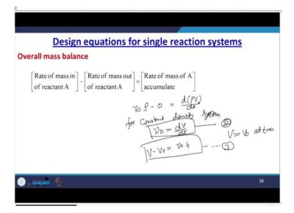
Now, if we try to write the overall mass balance, then we can write like this was the density. So, for the constant density system this can be represented as like this. Now, if we differentiate with initial concentration say at the start that V was V<sub>0</sub> and at time t = 0. So, we may have V - V<sub>0</sub> is equal to this one, let us put forward as equation number 3.
