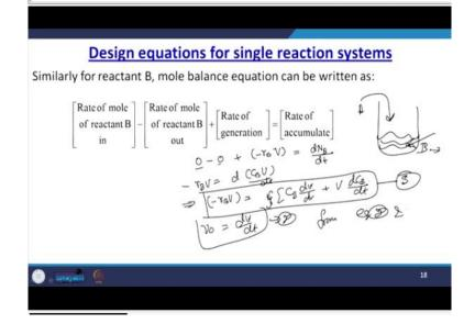
Now similarly for reactant B; because if you recall that one reactant was within the reactor and other was slowly added to that particular reactor, so, this was your A and this is the B. So, for the other reactant the mole balance equation you can easily write and that is your generic mole balance equation that is a rate of mole of reactant be in and whatever it is coming out plus the rate of generation is equal to rate of accumulation.
