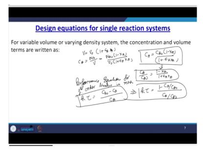
So, this is the basic approach for the graphical representation of mixed flow reactor. Now, for the varying volume system or the varying volume or varying density system, the concentration and volume terms you can write like this  $V = V_0 (1 + \text{epsilon A } X_A)$ .
