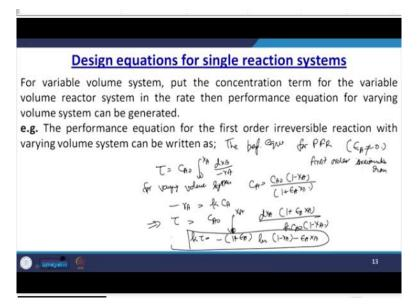
Now, the performance equation for PFR where we have this, that is the first order irreversible reaction. So, tau =  $C_{A0} dX_A$  Now, for varying volume system  $C_A = C_{A0} (1 - X_A)$  upon  $(1 + epsilon A X_A)$ .
