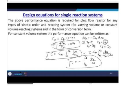
And plug flow system the reactants usually are consumed and converted into the product usually as it moves through the reactor length and the final conversion cannot end at the output of that reactor. So, if we try to integrate the things the previous this particular differential equation and for the whole reactor volume so, the final conversion if we are interested in the final conversion  $X_A$ .
