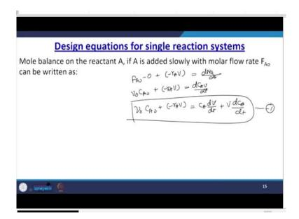
This can be written as  $F_{A0} - 0 + -r_A V = dN_A$  and dt. So, with respect to the concentration we can write like this. So, if you differentiate the above equation and try to rearrange the things, we may have this final equation  $C_A V dV dt$  plus this one d  $C_A dt$ . So, let us put this equation as equation number 1.
