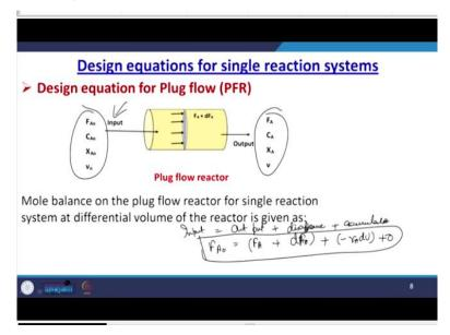
Now, this is our general PFR. Now, mole balance if you write the mole balance equation on the plug flow reactor for a single reaction system at various differential level. So, we can easily write that input is equal to output plus disappearance plus accumulation. Now, this can be written as  $F_{A0}$  based on this particular approach  $F_{A0} = F_A + \text{rate of disappearance - } r_A dv + 0$ . So, this is my basic equation or the mole balance equation for this particular approach.
