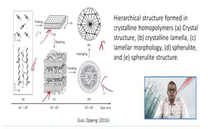
Now this is one particular hierarchical structure usually formed in the crystalline homopolymer. You can see that sometimes these are the crystal structures formed and then this is the crystal lamellae and then this is the lamellar morphology and spherulites you can see over here this is spherulite structures, etc. So, this is you can see just to visualize that what is the impact of different type of morphological approach in polymer system.
