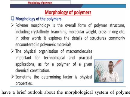
Now let us have a brief outlook about the morphological system of polymers. This is the overall form of a polymer structure. It includes the crystallinity, branching, molecular weight, molecular weight distribution, cross-linking, etc. So, in other word it explores the detail of structure commonly encountered in the polymeric materials and thereby it plays a vital role while the end use of those polymer which you synthesize in due course of time.
