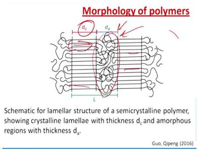
Now here you can see this is the schematic diagram of lamellar structure of semicrystalline polymer. This shows the crystalline lamellae with the thickness of d<sub>c</sub>. This is the thickness and amorphous region with the thickness of this one. So, you can see you can visualize the things they are entangled in nature and they are you can see they are having the regular array in this one.
