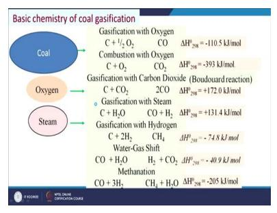
So, this is the basics of the gasification process now we will see the chemistry, the reactions what happens in whatever reactions takes place in case of gasification process, so we have here feedstocks coal we have oxygen and we have steam. Now these schemes show us the elemental reactions the coal is having carbon it is having hydrogen it is oxygen, sulphur, nitrogen etcetera but we are considering the major components of the coal that is carbon we are considering in this case.
