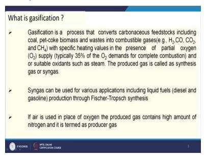
And the syngas can be used for various applications including the liquid fuel production through the Fischer-Tropsch synthesis and if air is used in this process in place of oxygen then the syngas contains more amount of nitrogen and that is called a producer gas.
