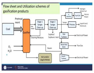
Now we will see that how we will use this, the flowsheet and utilization schemes of gasification products. So, we have coal here then we are sending it to gasifier with steam and oxygen then we will get syngas. So, syngas has to be cleaned up first, the first stage of cleaning so we are
