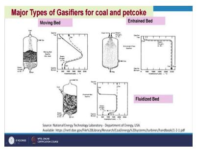
So, on the basis of the feed inlet gas collection and the operating conditions different types of gasifiers are reported out of which moving bed, fluidized bed and entrained bed are the major 3 important gasifiers which have been used widely for the gasification of coal and other carbonaceous feedstocks. In the moving bed coal is feed at the top and the particle size is higher say 5 to 50 millimetre particle size.
