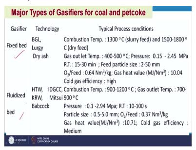
So, fixed bed, fluidized bed you see these are the technology licensers BGL, Lurgy, dry ash that is the fixed bed and HTW, IDGCC and KRW and Mitsui Babcock. So, these are the technologies licensers and typical process conditions for these are the combustion temperature is 1300 centigrade and slurry feed if it is and if it is a dry feed then 1500 to 1800 °C. But gas outlet temperature is less 400 to 500 °C and pressure is this much and particle size already discussed.
