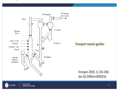
So, that is why transport reactor gasifier has been developed by KBR so in this case we have the intermediate properties both the fluidised bed and entrained bed properties are available here how? We are putting here fuel then absorbent we are putting some adsorbent also that is to capture the sulphur and then oxygen or air and steam all are here in coming into this reactor. Then it is going up this riser section very small time it is getting for contact.
