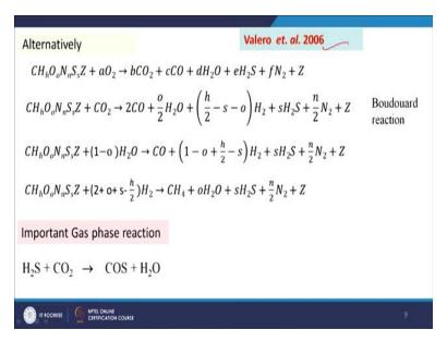
So, tars will be available with this. In 2006 Valero they have presented this phenomenon nicely considering the presence of ash as well as sulphur nitrogen etcetera they have given the molecular presentation of the coal that is  $CH_hO_oN_nS_sZ + aO_2$  and this is converted to  $CO_2$  CO  $H_2O$   $H_2S$   $N_2$  and Z, Z is our ash. So, this is the reactions they have proposed and they have shown the mass balance and how to calculate a; how to calculate h o n s Z etc.
