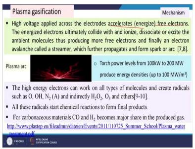
Now we will see the advanced process in gasification's, the plasma gasification is one of the advancement in the gasification process, in this case we use high voltage across the two electrodes. So, in that case the electrons are emitted then electron accelerates free electrons electrodes accelerates free electron and free electrons helps to oxidize or ionize the ions adjacent ions and molecules and then number of electrons are produced which forms a avalanche that is called streamer.
