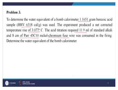
Now, we are coming to problem number three. The statement is; to determine the water equivalent of a bomb calorimeter 1.1651 gram benzoic acid sample high heating value 6318 calorie per gram was used. The experiment produced a net corrected temperature rise of 3.077 °C the acid titration required 11.9 ml of standard alkali and 8 centimetres of Parr 45C10 nickel-chromium fuse wire was consumed in firing. So determine the water equivalent of the bomb calorimeter.
