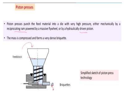
Now we will see the piston press. So here the figure shows the piston press. So this is the piston, so here if we put the feedstock, so feedstock under gravity it will go down and when it will come entering here, so this piston will have back and forth movement and this will be pressed here. So this, we are getting the briquette. So here, the piston can give us very high pressure. So the density of this material will be very high with respect to other method.
