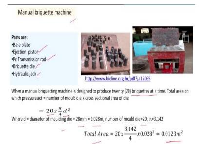
Then we will see the manual briquette machines which are used in small scale, they are small machines and anybody can use it easily. So, here different parts are there. We have one base plate. So, these are base plates and base plates will having some ejection piston. So, if we see here, we have one hydraulic jack here. So, then the pistons are there, and ejection pistons and transmission rod.
