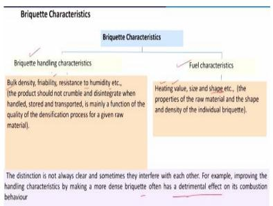
Now briquette characteristics. There are some properties the briquette should have because briquettes have to be transported from one place to other place. So, one will be there is handling characteristics and another will be fuel characteristics. Our main objective for the production of briquettes is to get energy from it, so use it as a fuel in combinations. So heating value, size and shape.
