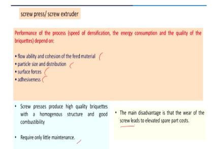
Now, the performance of the process will depend upon some factors that is your the ability and cohesion of the feed material, then the particle size and its distribution, surface forces and adhesiveness. So, these are the factors which influence the performance of the process. The screw presses produce high quality briquettes, this also produce high quality briquettes with a homogeneous structure and good combustibility and require only little maintenance.
