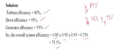
Now let us move to problem number 3. So it says for a typical small hydro system water flows through a head of 2.5 meters and a turbine that could take a maximum flow rate of 3 meter cube per second. If the turbine efficiency would be 85%, drive efficiency 95% and
