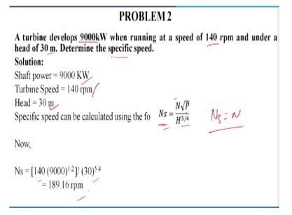
Now we are moving to problem number 2. The statement is a turbine develops 9000 kilowatt when running at a speed of 140 rpm and under a head of 30 metre. Determine the specific speed. So this is again a problem related to hydro turbines and here we have to define the specific speed. So, specific speed is nothing but the speed which is equivalent to a turbine having the same sides and that turbine which can produce unit power by using unit head.
