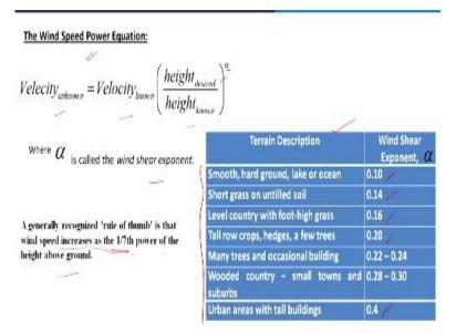
The other expression which is used to predict the wind speed at any height if we know the wind speed at any other height that is equal to that is a power equation, so velocity at unknown = velocity of known x height of desired and then height of known, so height desired means that is for unknown and this is for known velocity and height and then to the power alpha, that is a power expression.
