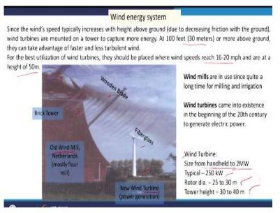
Now we will see the wind energy systems. So here, this figure shows us 2 systems, one is your old windmill and another is a new wind turbine. So old windmill we have brick tower where in both the cases we see the blades or the rotor is placed at certain elevation, so not at the immediate surface of the earth, it is put at certain height. So the height is required because as you go up the wind velocity increases.
