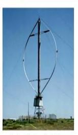
Vertical axis type wind mill
