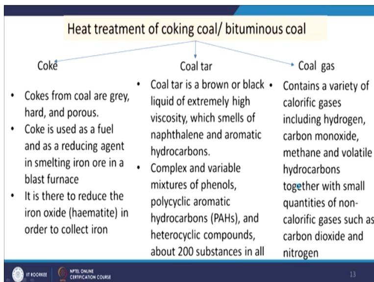
Now in thermal power plant we produce flue gas by the combustion of coal in presence of air, but if we do not apply air, just heat it in absence of air, then coal will be converted to three products, one is your coke and others coal tar that is liquid and another coal gas. So, solid liquid and gas will be getting, this coke which is produced here that will be having superior quality with respect to coal and can be used for steel production.
