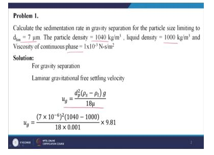
As for this formula that is terminal settling velocity is equal to dp square into  $\rho_s$  minus  $\rho_l$  into g divided by 18 into  $\mu$  when dp is the diameter of the particle,  $\rho$  s is the density of the solid particle  $\rho_l$  is the density of the fluid under which the particle is falling g is the acceleration due to gravity gravitational acceleration and then  $\mu$  is the viscosity of the media. So, we have to calculate ug.
