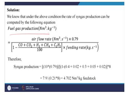
As we have discussed in the previous classes that fuel gas production normal meter cube per kg of feedstock that is equal to air flow rate normal meter cube per second into .79 divided by 1 minus the  $CO + CO_2 + H_2 + CH_4 + C_2H_2$  there is the composition of the flue gas by 100 into feeding rate of the feedstock. So, feeding rate of feedstock this is the total amount we are using per unit time and then 1 – this.
