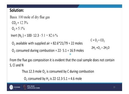
Now let us solve it so we are taking 100 mole of dry flue gas, this is our basis then what will be the CO<sub>2</sub> as it is 12.3% and O<sub>2</sub> 5.1% so this 12.3 moles and 5.1 moles it will be an inert will be rest of it. So, 100 - 12.3 - 5.1 that is equal to 82.6% so 82.6 moles will be so oxygen available with supplied air that is equal to how much 82.6 so we are assuming that 21% oxygen rest is nitrogen so this into 21 divided by 79.
