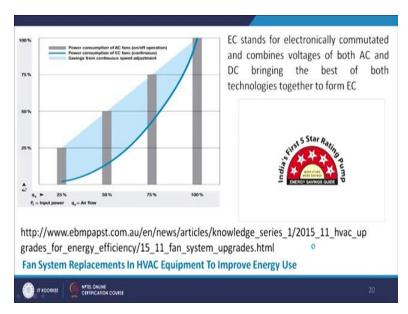
Another example is your power consumption of AC fans and EC fans. If we compare, so this is our EC fan power consumption and here this is AC. So, this much of energy we can save. how it is possible? By the improvement in the technology, you see here EC stands for electronically commutated and combines voltage of both AC and DC. Bringing the best of both technologies together to form EC, another is we are talking about the regulations and guideline.
