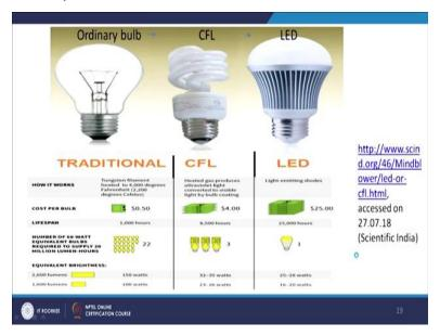
So, already people are working on this, so new technologies are being developed which are more efficient in terms of energy efficiency. So, here some example is traditional bulb, ordinary bulb, and CFL and LED. See, compare these three types of technologies, then we see cost is different we also see to give same amount of intensity of light different number of bulbs are required. And their lifespan is also different.
