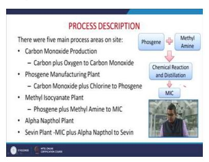
Now, let us have a look about the process description, so there were five main process arena, carbon mono oxide production with the help of carbon plus oxygen to give the carbon monoxide, the second was the phosgene manufacturing unit this the carbon mono oxide plus chlorine to produce the phosgene then they were having the MIC plant that is phosgene plus methylamine to
