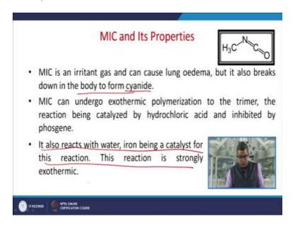
Now, this MIC is an irritant gas and can cause the lung edema but it also break down in the body to form the cyanide, so the root of this breakage is again important and because it was the root
