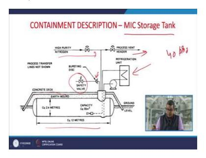
So when it was entered into the storage tank, so let us have a containment description that is the MIC storage tank. Now this MIC storage tank was having the diameter of 2.5 meter the length of 12 meter, it is duly supported by the safety valve with the busting disc, this is equipped with the refrigeration unit. It is having the ground level concrete deck and we have already discussed that
