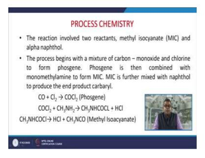
So basically the reaction involved two reactants methyl isocyanate and alpha naphthol the process begins with the mixture of carbon monoxide and chlorine to produce phosgene and phosgene is then combined with mono methyl amine like in this particular slide to form MIC. Now MIC is further mixed with naphthol to produce the end product carbonyl. So this was the entire stream and the chemical reactions are given in this particular these lines.
