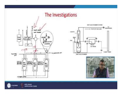
So this was the thing like this was the vent gas scrubber cost with the caustic and this was the relief valve head the vent header. So he was trying to clear the any kind of possible choke and in these lines, but he forget he probably he forget to insert a blind within this system.
