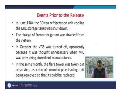
In June 1984, about 10, about 30 ton refrigeration unit cooling the MIC storage tank was shut down and the charge of the Freon refrigerant was drained from the system. The again the reason
