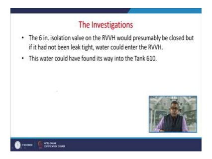
So a six-inch isolation valve on relief valve vent header would presumably be closed but if it had not been leaked tight water could enter the RVVH. So it was mandatory at the time that either the blind or a blank should be inserted because if this isolation valve is not tight enough then water may enter into the tank 610, so water, so by this way, the water could have found its way into the tank number 610.
