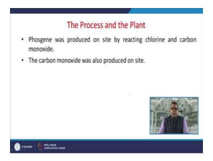
So phosgene was produced on site by reacting chlorine and carbon mono oxide and this carbon monoxide was also produced on site. So that is why when the initially whatever gas was leaked the prima facie formation provided by Union Carbide to the local authority that it is chlorine. So the treatment of chlorine and is entirely different with methyl isocyanate. So we will discuss this particular aspect in due course of time.
